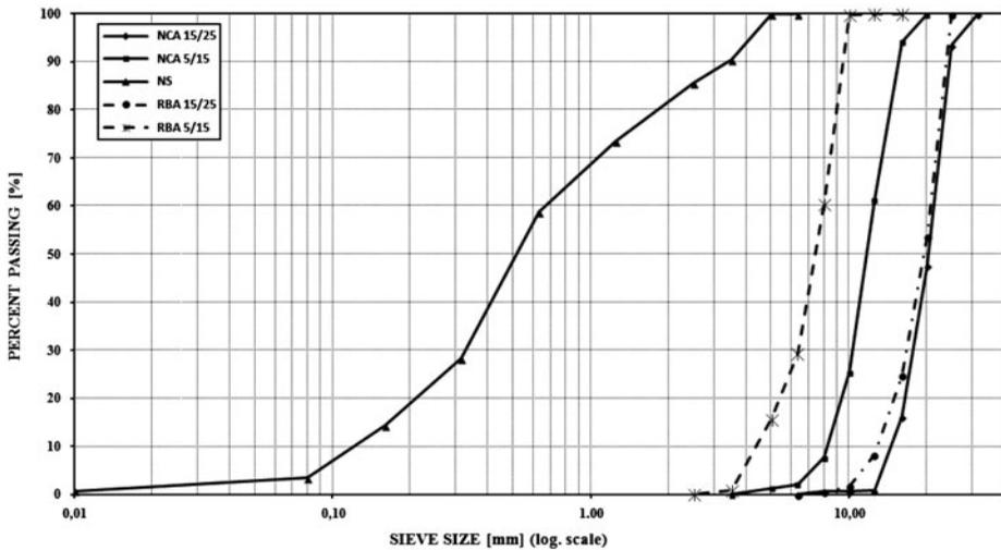
Figure 1. Grading of natural and recycled aggregates.
