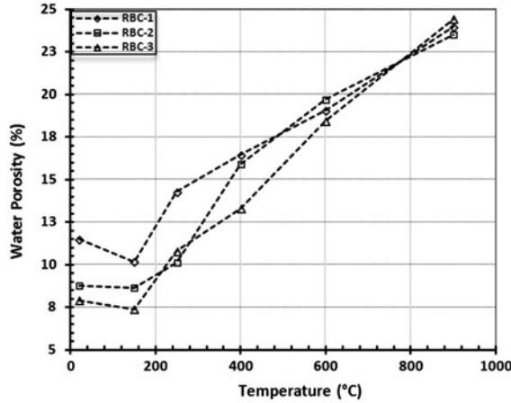
Figure 8. Water porosity of RBC specimens after exposure to elevated temperatures.
