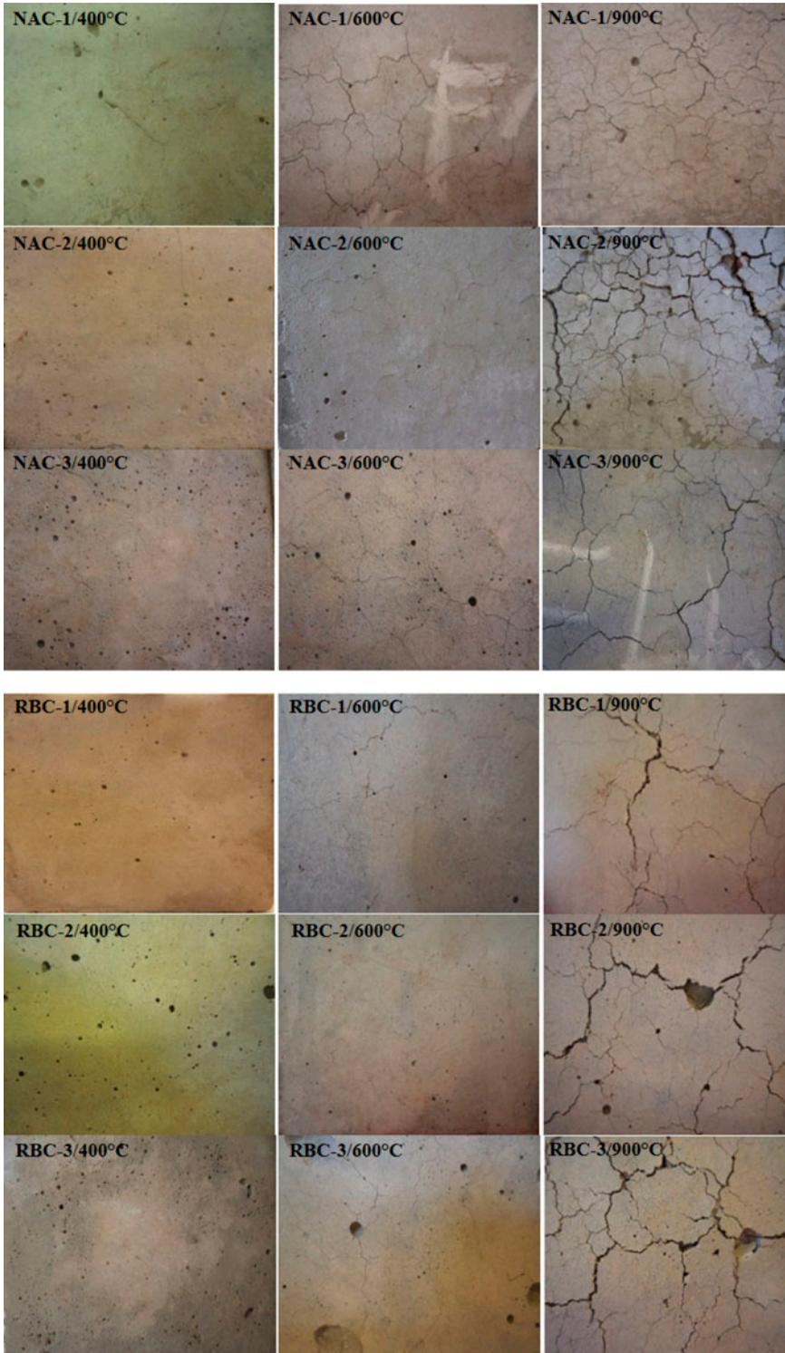
Figure 12. Typical crack patterns observed in NAC and RBC at 400, 600 and 900 °C.
