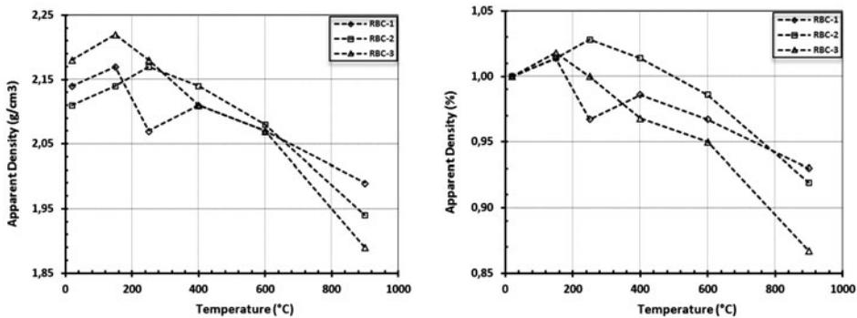
Figure 9. Residual density of RBC specimens after exposure to elevated temperatures.
