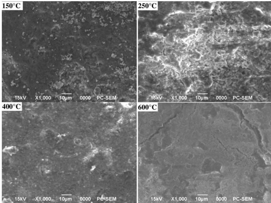
Figure 11. SEM micrograph of surface microstructure of RBC-3 exposed to elevated temperature (scale bar 10 µm).
