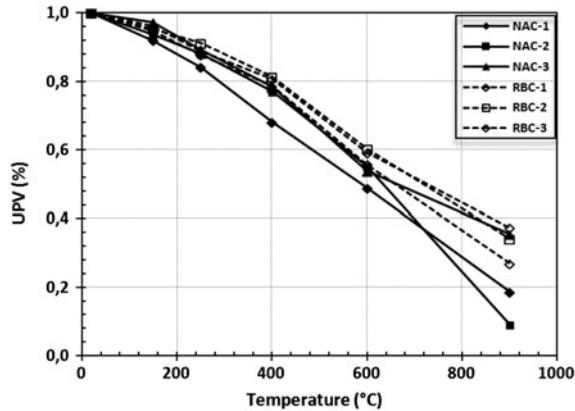
Figure 6. Relative UPV as a function of elevated temperature.
