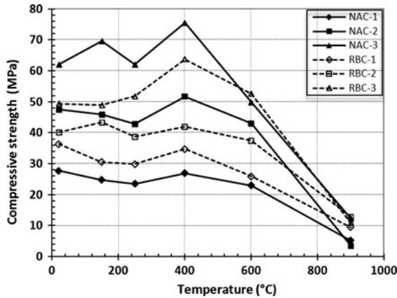
Figure 3. Residual compressive strength of NAC and RBC after exposure to elevated temperature.
