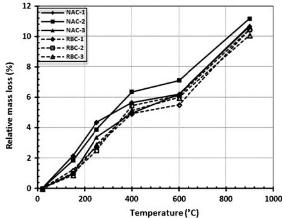
Figure 7. Mass loss of the NAC and RBC specimens subjected to elevated temperature.
