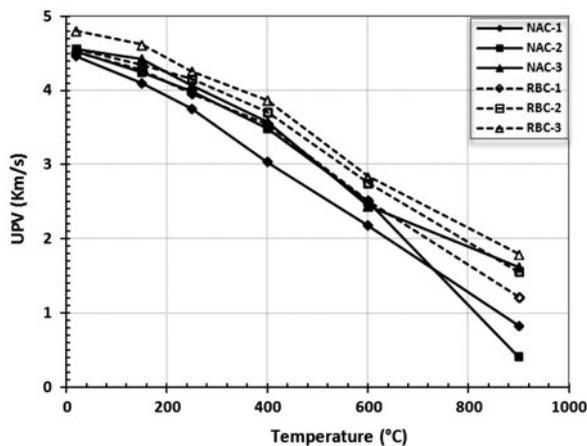
Figure 5. UPV as a function of elevated temperature.
