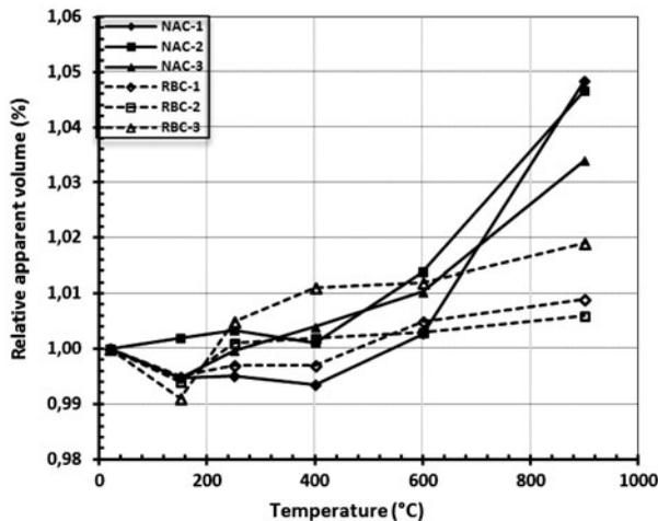
Figure 10. Relative volume of NAC and RBC specimens as a function of elevated temperatures.
