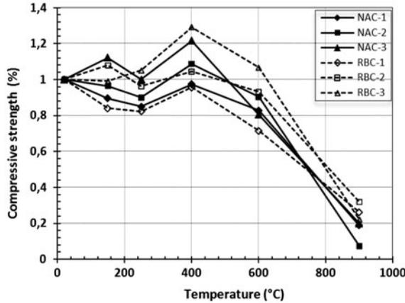
Figure 4. Relative residual compressive strength of NAC and RBC after exposure to elevated temperature.
