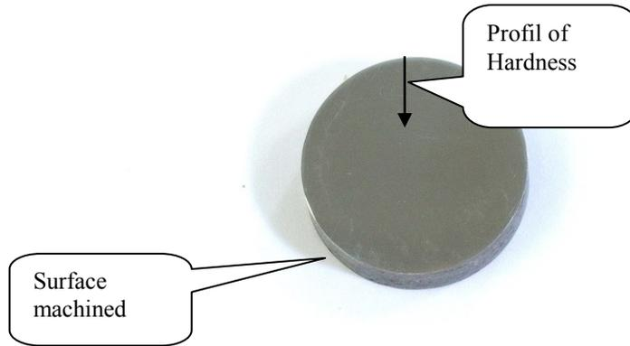
Figure 3 : Specimen of machined XC18 steel.
