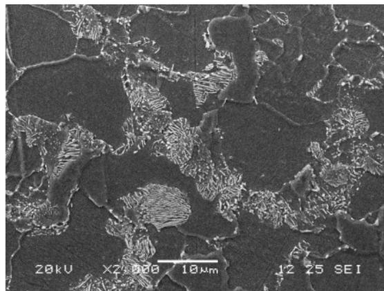
Figure 4 : Microstructure of low carbon steel (AISI 1055)
