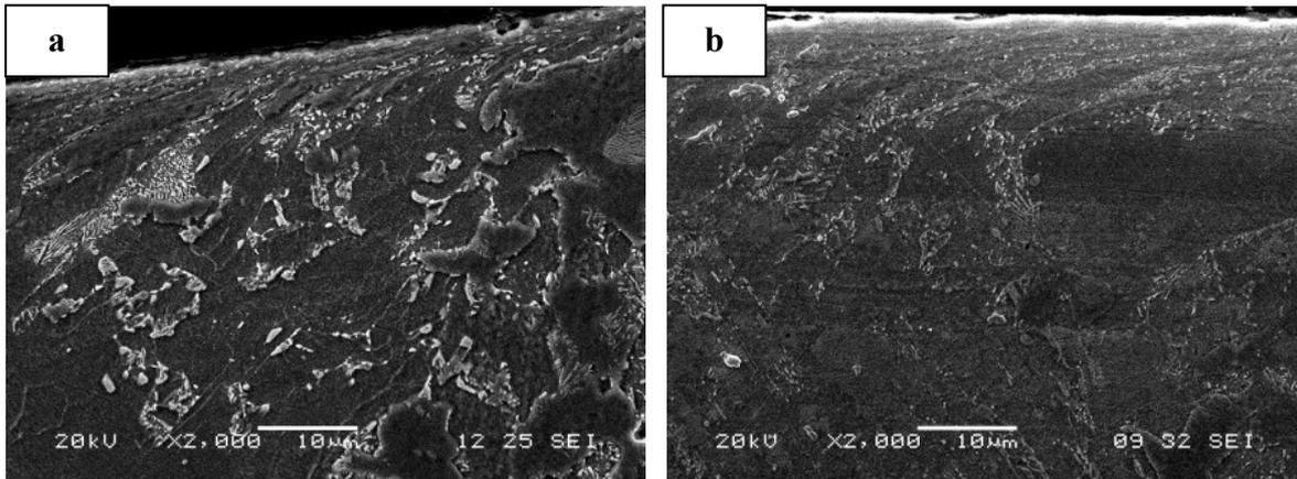
Figure 5 : Microstructures of the cross-section of low carbon steel after two cutting speeds by hard turning : (a) V2 = 560 and (b) V4 1100
