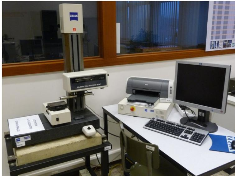
Fig. 2 Photographic view of the surface roughness tester.
