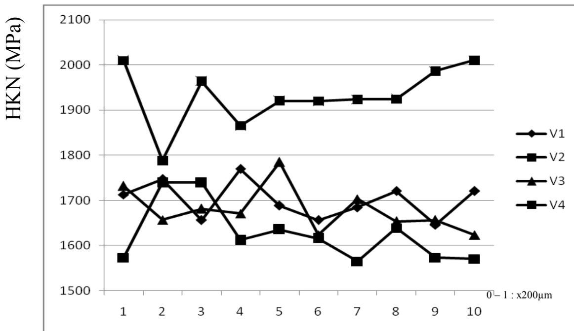
Figure 6 : Knoop hardness evolution curves from the surface to the core of low carbon steel after different cutting speed by hard turning.
