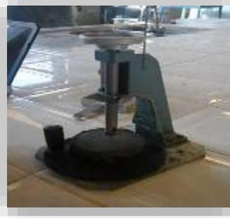
**Figure IV.14:** Appareil de consistance Vicat
