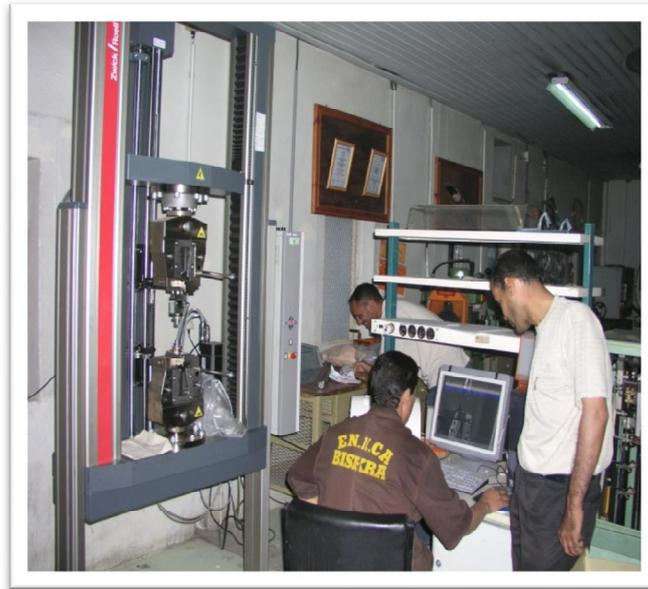
**Figure IV.6 :** Machine de traction de type Zuick/Roell Z 100.
