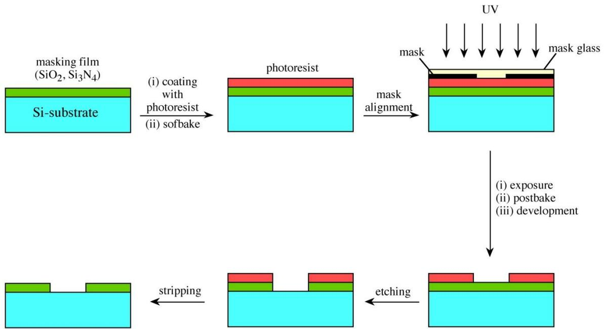
**Fig.II.2** Steps in optical printing using photolithography [10].
