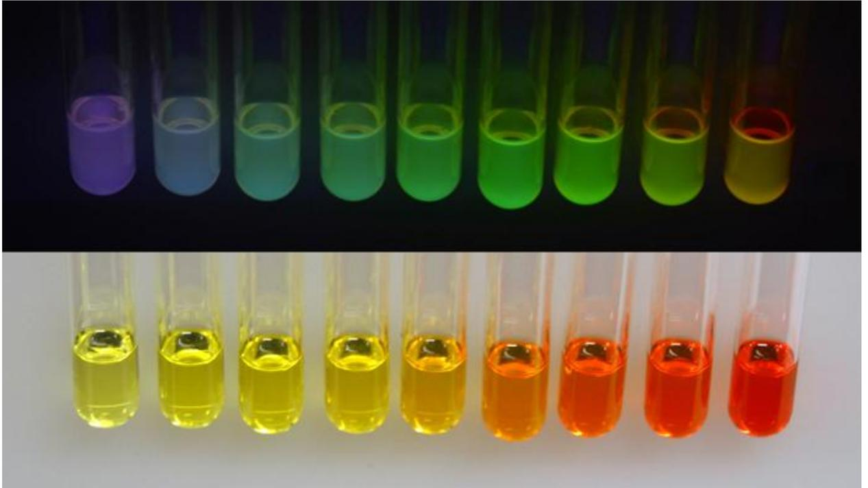
**Fig.III.1** Top: Long wave UV illumination. Bottom: Ambient illumination. Solutions are in order of increasing particle size (longer growth time).
