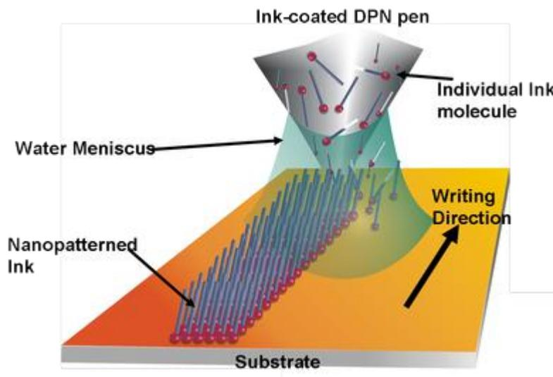
**Fig.II.4** schematic drawing of the Dip-Pen Nanolithography (DPN) technique [14]
