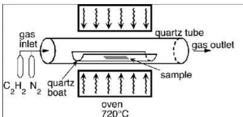
Fig.II.5 Schematic diagram of the chemical vapor deposition apparatus [18].
