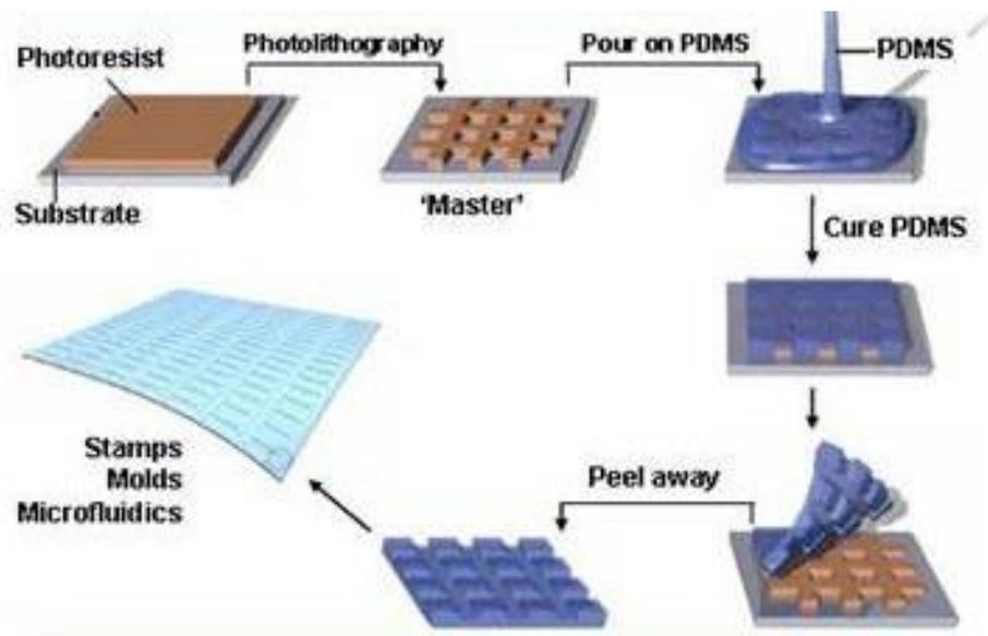
Fig.II.3 Schematic illustration of the procedures for fabricating soft lithography [12]
