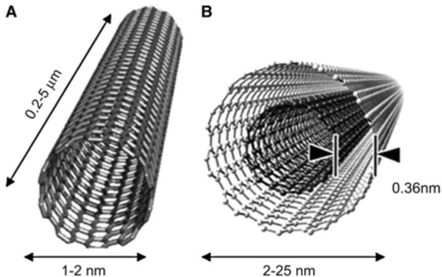
**Fig.III.2** conceptual diagram of single-walled carbon nanotube (SWCNT) (A) and multiwalled carbon nanotube (MWCNT) (B) delivery systems showing typical dimensions of length, width, and separation distance between graphene layers in MWCNTs [21].
