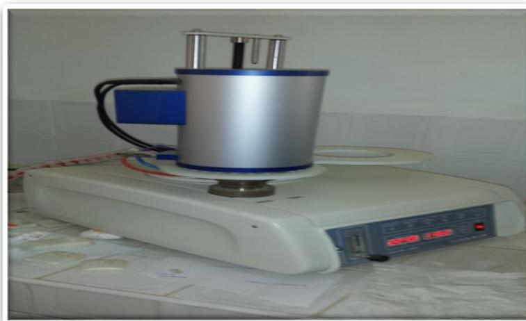
**Figure II.5:** Appareil Couplage ATD/.ATG
