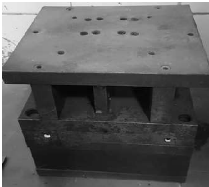
Figure IV-5 Crevice Corrosion of steel die mold.
