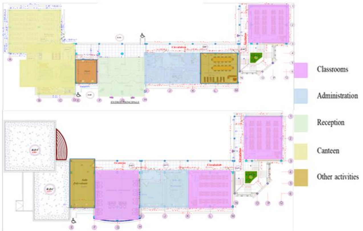
Picture 32: a) Spatial organisation on the ground floor /b) Spatial organisation on the first floor
