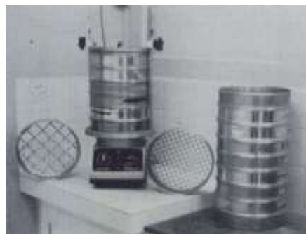
Fig 26. Check the Condition of Sieves
