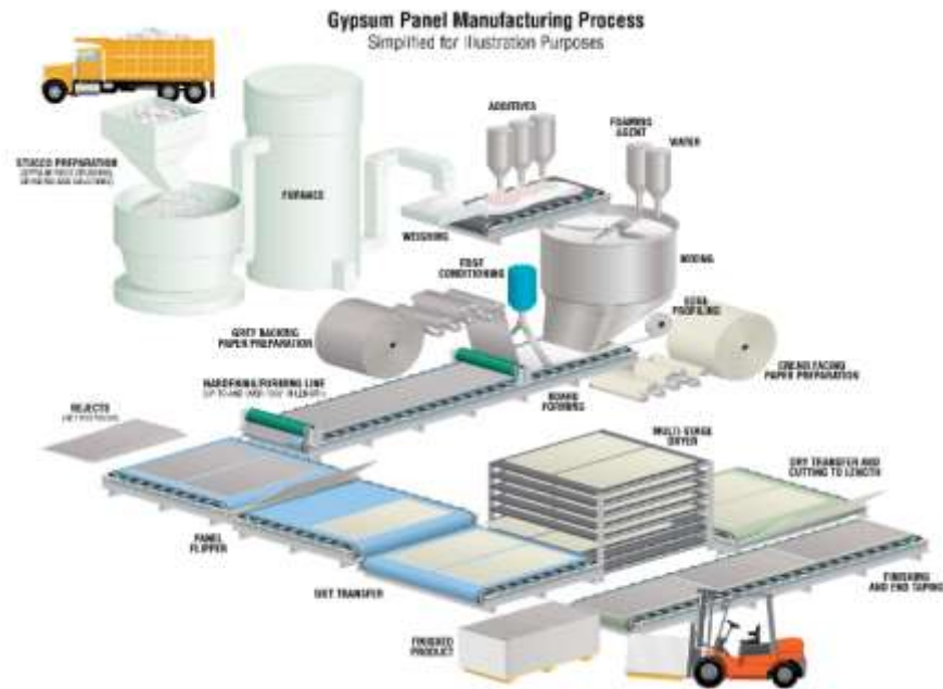
Fig 11. Gypsum panel manufacturing process
