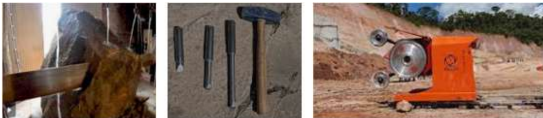
Fig 45. helical wire sawing, and the use of steel wedges
