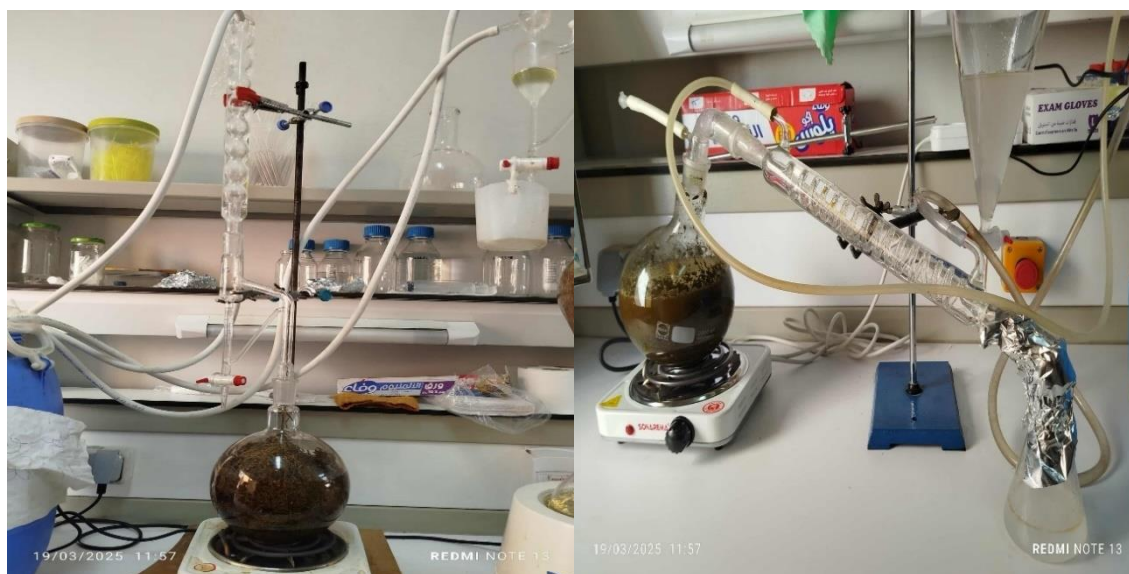
Figure 9: Clevenger type apparatus used for hydrodistillation
