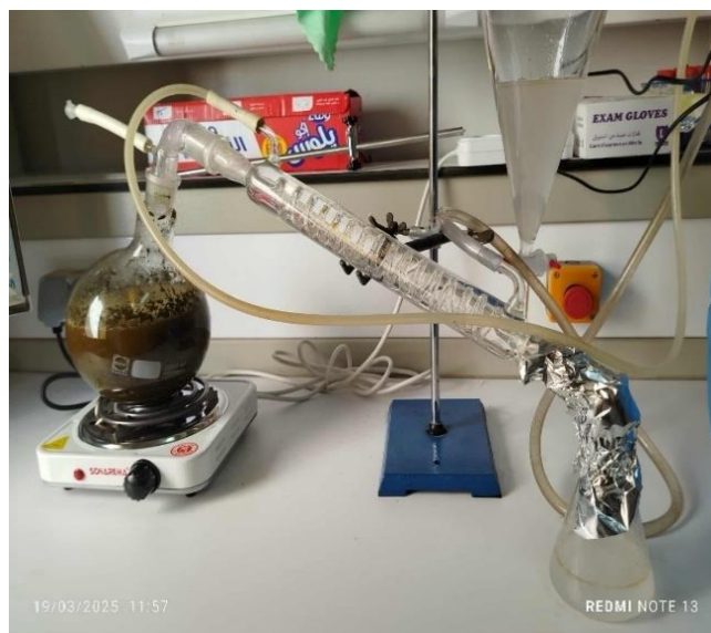
Figure 2: Clevenger type apparatus used for hydrodistillation
