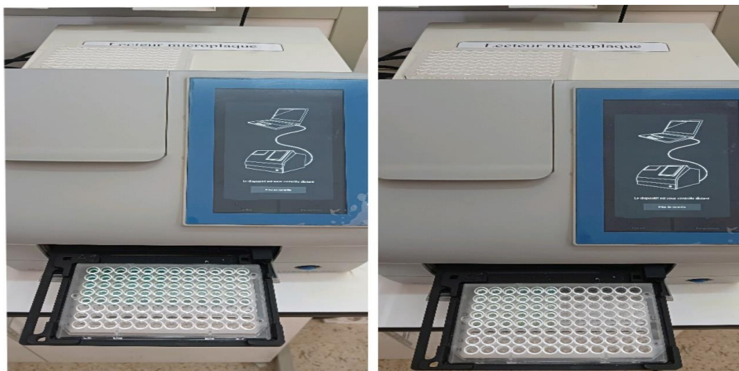
Figure II.9: Spectrophotometer for measuring antioxidants activity (phenanthroline assay)
