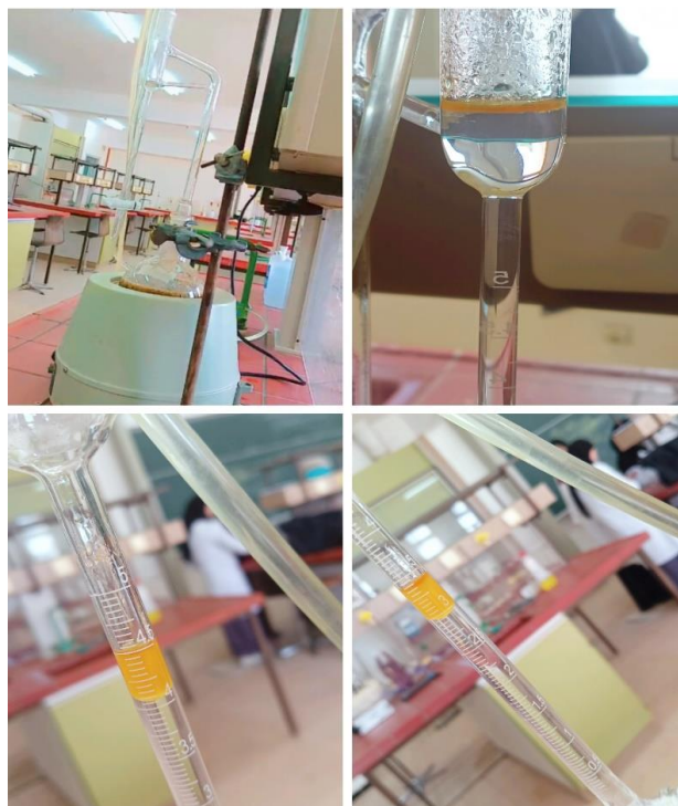
Figure II.2: Clevenger Apparatus for Essential oil Extraction
