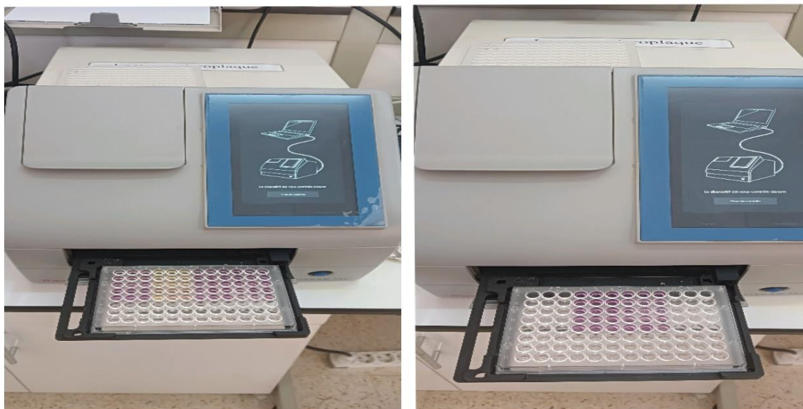
Figure II.5: Spectrophotometer for measuring antioxidants activity (DPPH assay)
