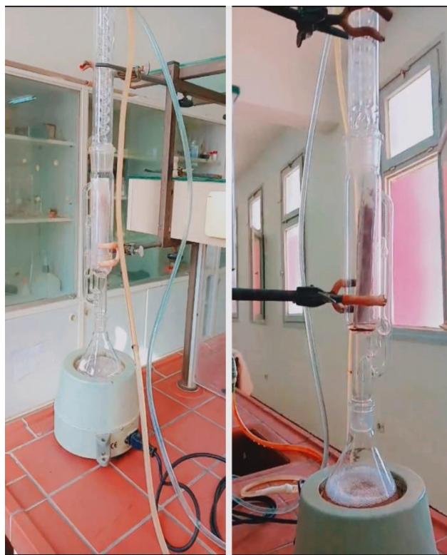
Figure II.1: Soxhlet Apparatus for Extracting plants oils
