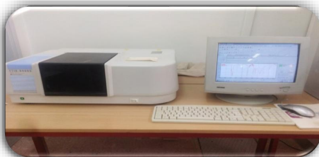
Figure II.7. Fourier-Transform Infrared Spectrometer
