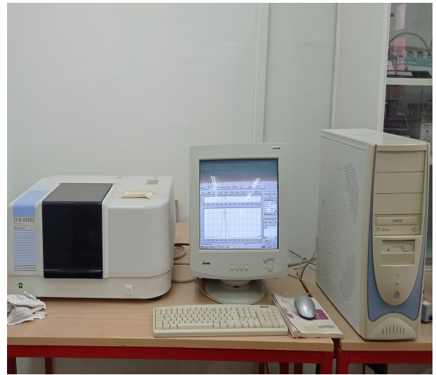
FIGURE III.19 spectrophotomètre SHIMADZU – FTIR 8400S.
