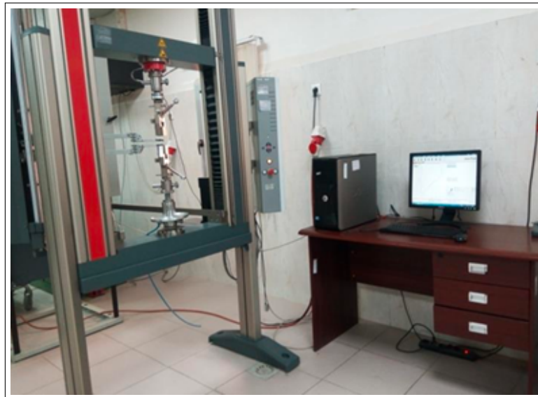
FIGURE III.15 Machine de traction de type Zwick/Roell Z050.
