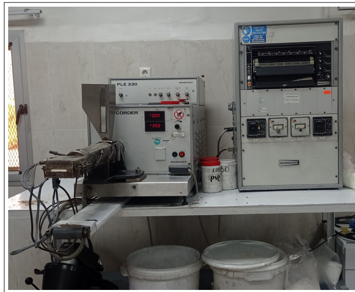
FIGURE III.11 Extrudeuse de type Plasti-Corder PLE 330.
