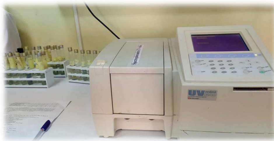
Photo 11 : Dosage de Phosphore assimilable (photo original).
