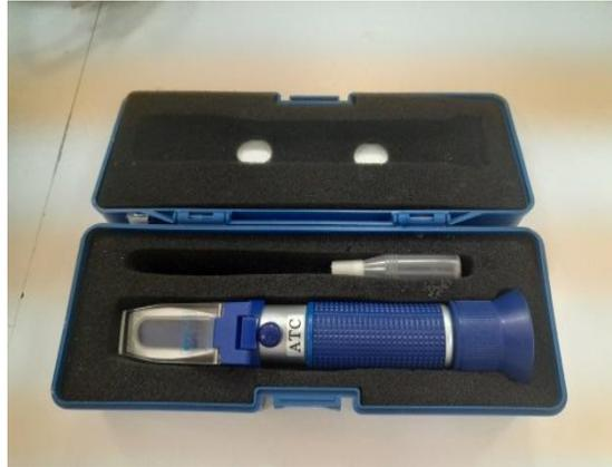
**Figure 3 : Refractometer**
