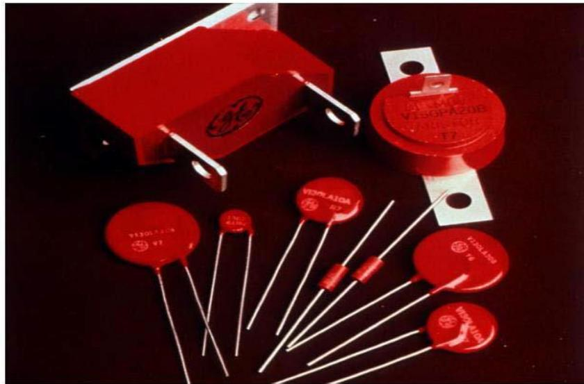
**Figure I. 13 : Different shapes and sizes of ZnO varistors for the protection of electrical equipment operate at voltages [91].**
