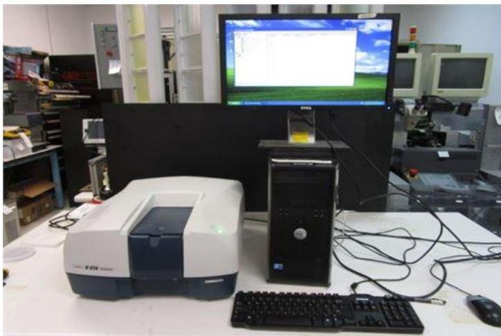
**Figure II.19: V-750 UV-Visible Spectrophotometer.**
