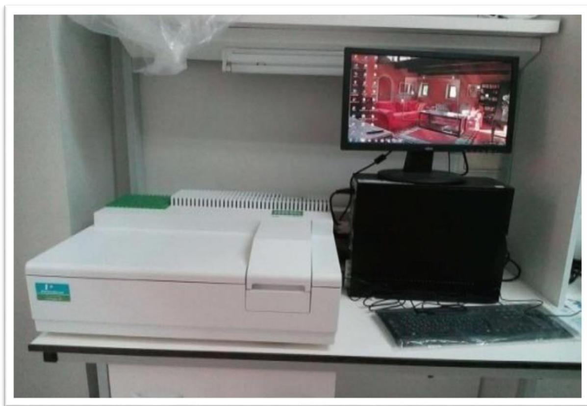
**Figure II.11:** Perkin Elmer Lambda 35 UV-Vis spectrophotometer.
