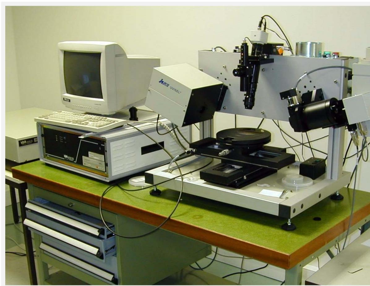
**Figure II.13:** Uvisel ellipsometer from HORIBA Jobin Yvon.
