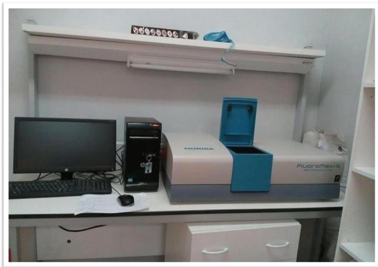
**Figure II.16:** Horiba Yvon FluoroMax®-4 spectrofluorimeter.
