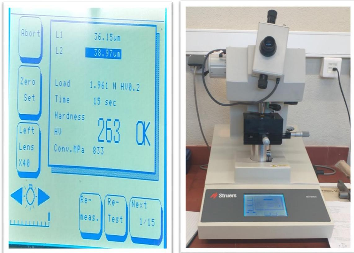
**Figure II.10:** Duramin struers of Vickers hardness.
