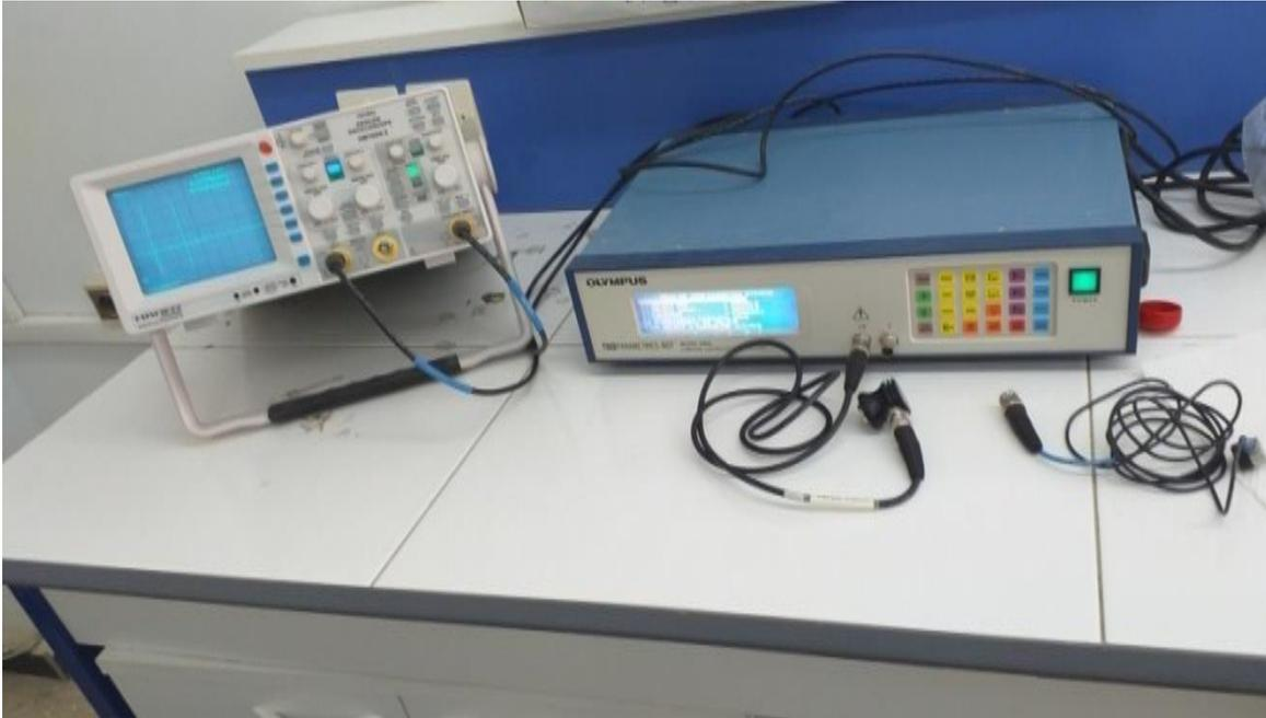
**Figure (II.9):** Pulse-Echo set up: Immersion transducer with Olympus Panametrics-NDT Model 5800 generator, coupled with an oscilloscope 20GHz (type HAMEG).
