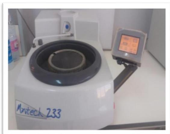
**Figure II.5:** type polisher Minitex 233 Megapol Pressi
