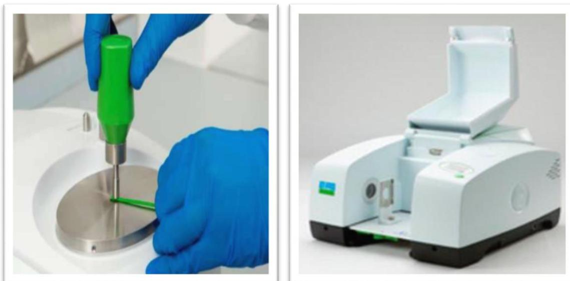
**Figure II.15:** a) UATR techniques of the Perkin Elmer spectrophotometer. Spectrum Two. b) Spectrum Two spectrometer (FT-IR).
