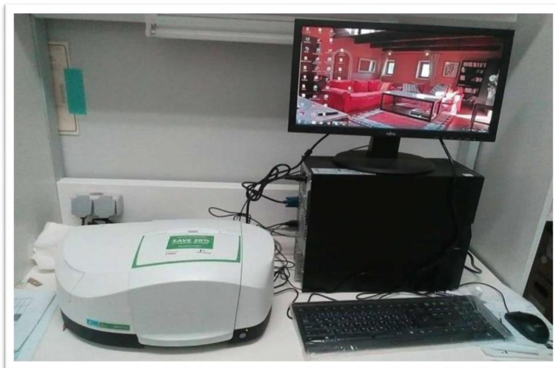
**Figure II.14:** Perkin Elmer Spectrum Two FTIR spectrophotometer.
