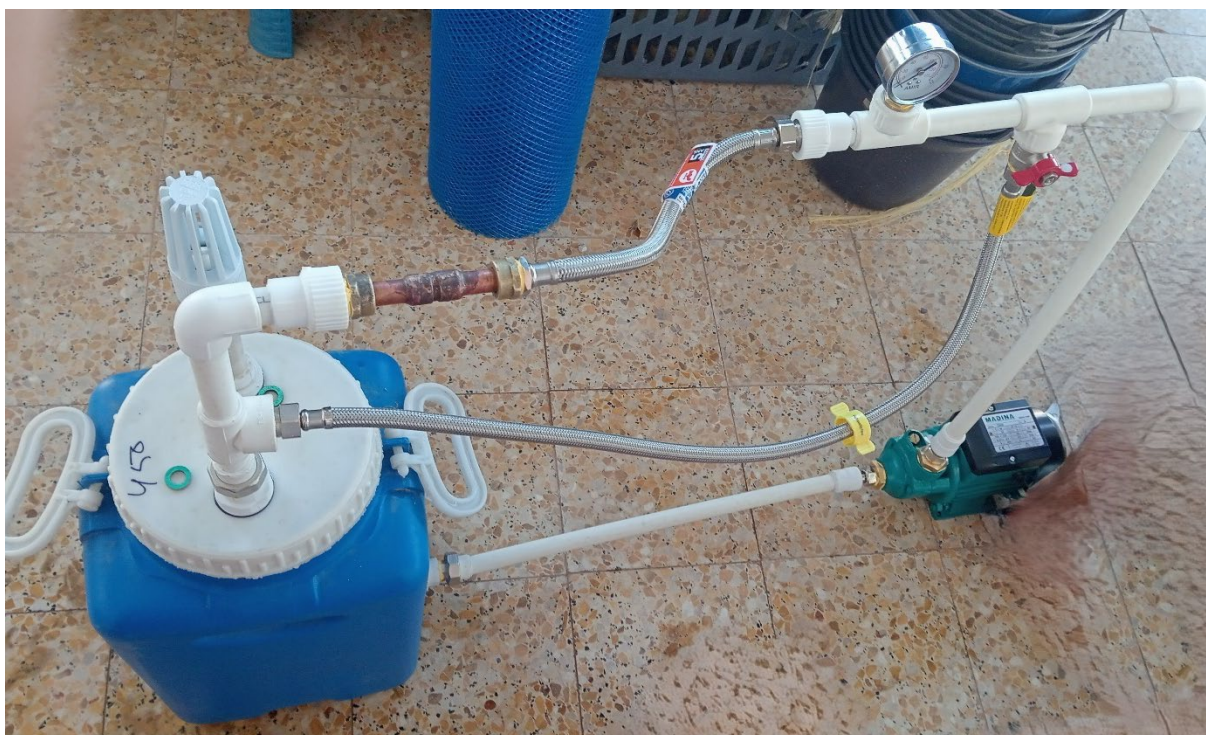
Figure IV.11 Custom Made Filtration Permeability Tester
