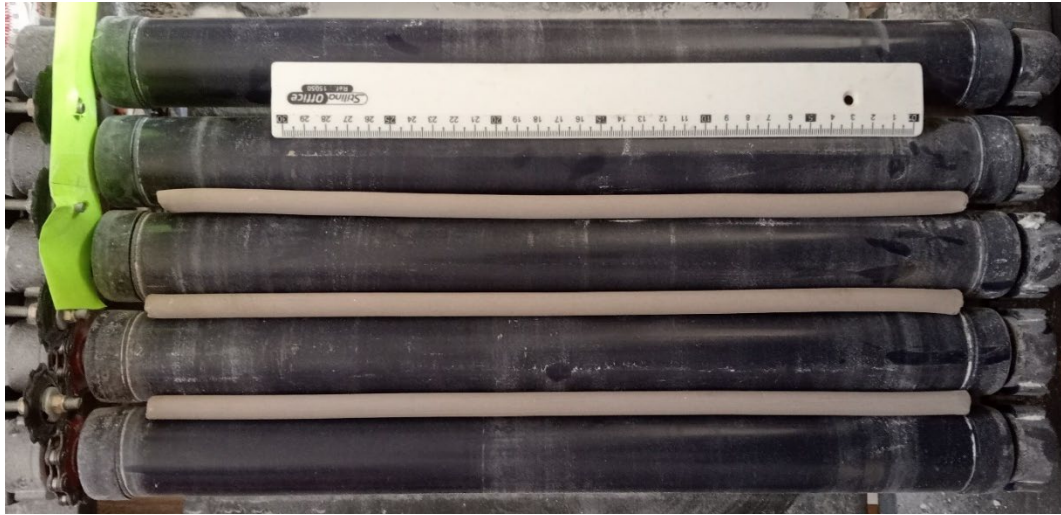
Figure III.8 Samples After the Initial Drying Process 30 cm Ruler for Reference
