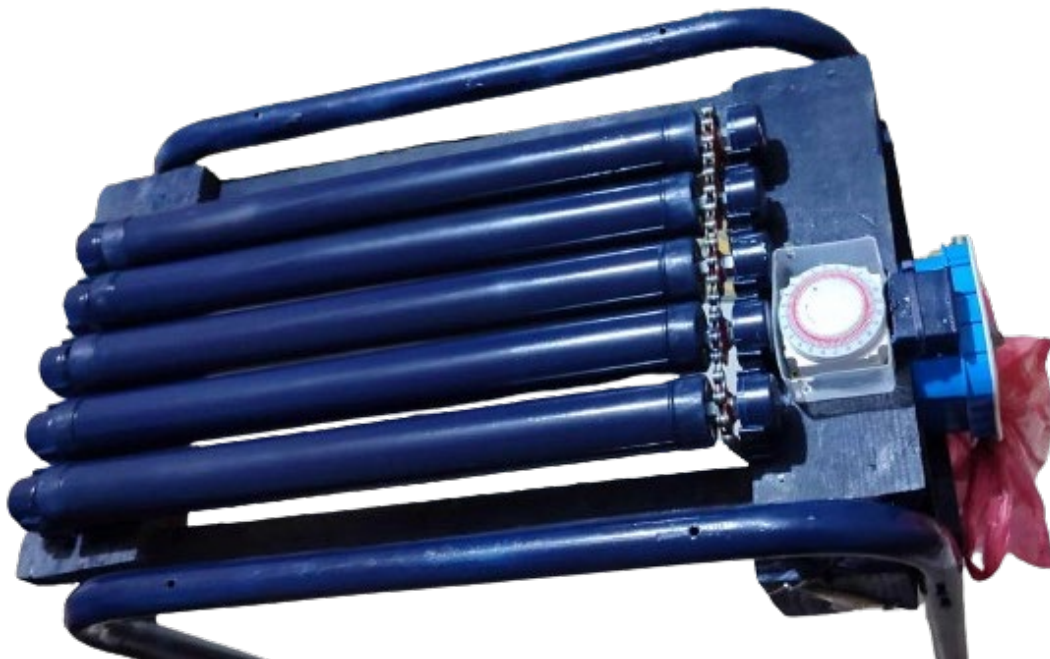
Figure III.7 Custom-Built Roller Dryer Table
