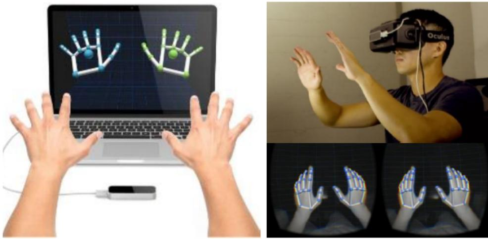
**Figure 3.10:** Leap Motion devices [24].
