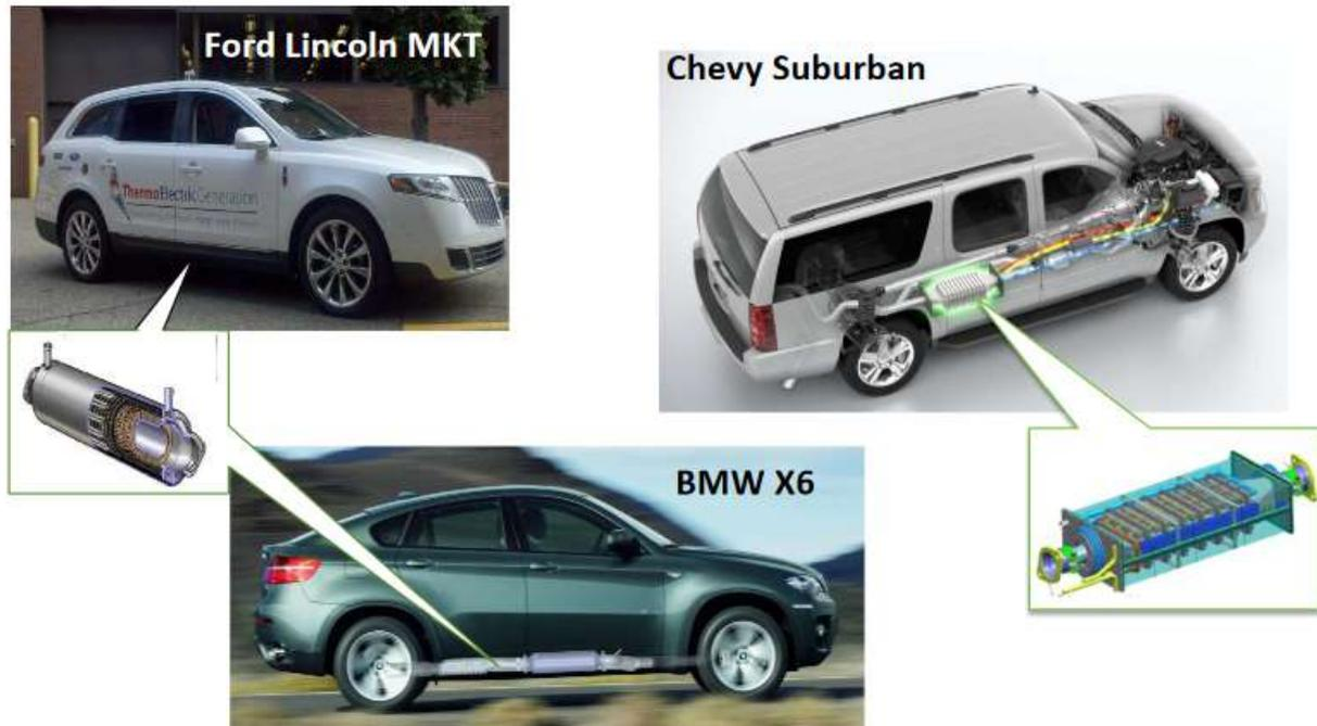
**FIGURE (I-9):**Vehicle Integration with Thermoelectric : FORD, GM and BMW Prototype integration pursued under DOE/industry sponsorship.
