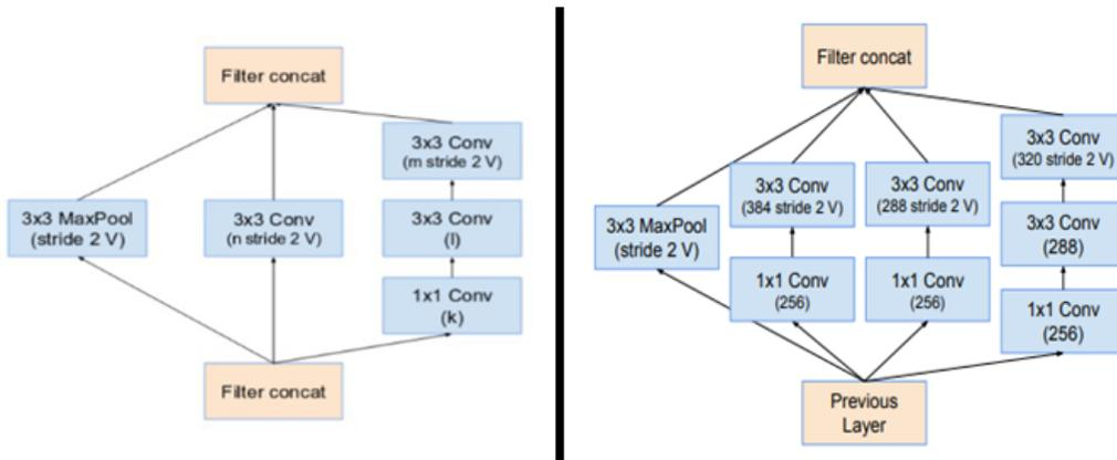
Figure 5.13: Reduction block A and B of InceptionResNetV2
