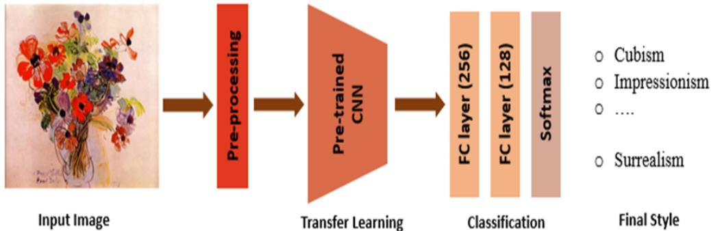
**Figure 5.1:** The proposed framework for style recognition
