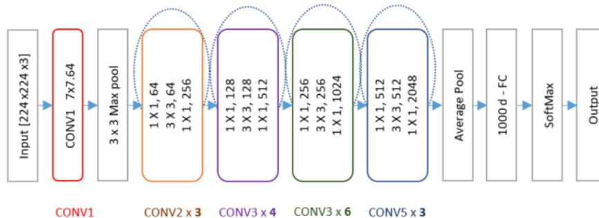
Figure 5.9: Architecture of Resnet-50
