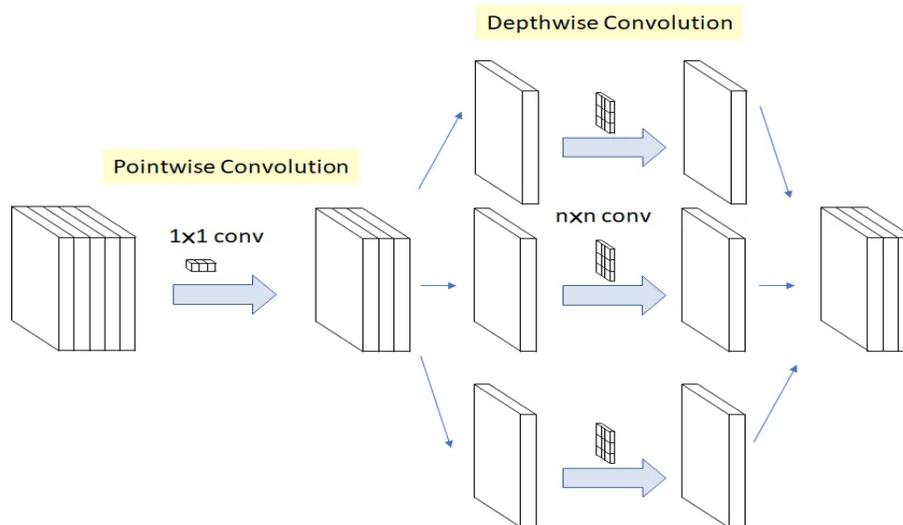
Figure 5.6: The depth-wise and point-wise convolution modules in the architecture of Xception
