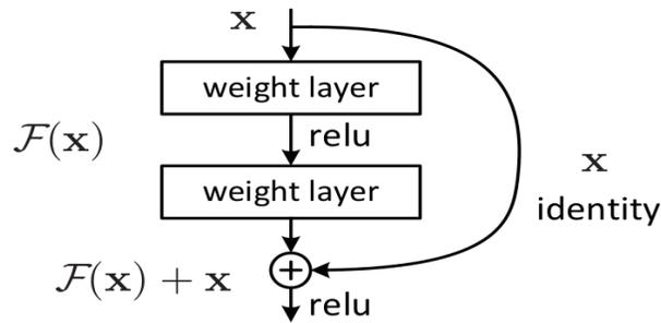
Figure 5.8: Residual connections
