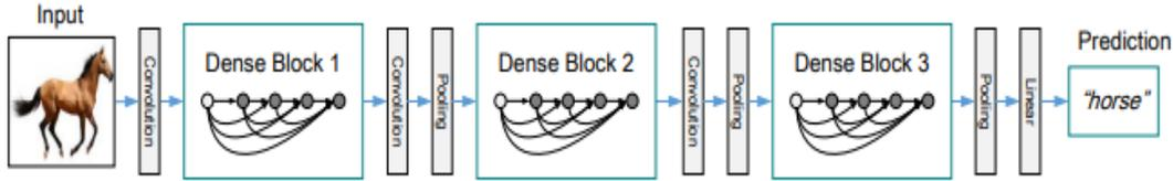
Figure 5.14: Architecture of DenseNet with 5 blocks
