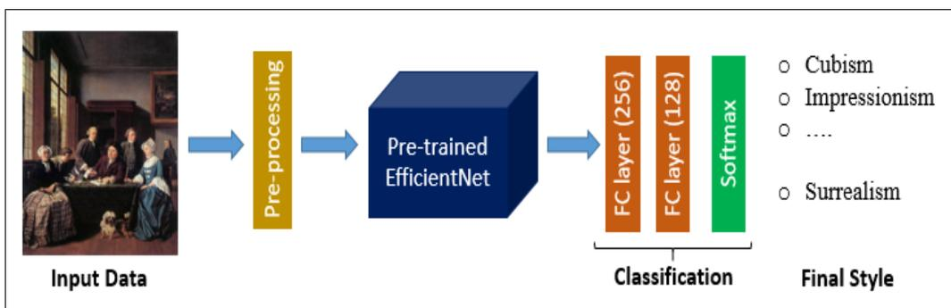
Figure 4.2: General framework of our custom pre-trained EfficientNet models for style classification
