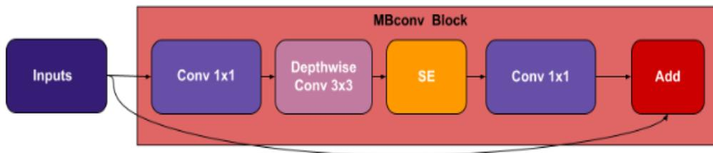
**Figure 4.9:** The MBConv block with SE block in the EfficientNet architecture
