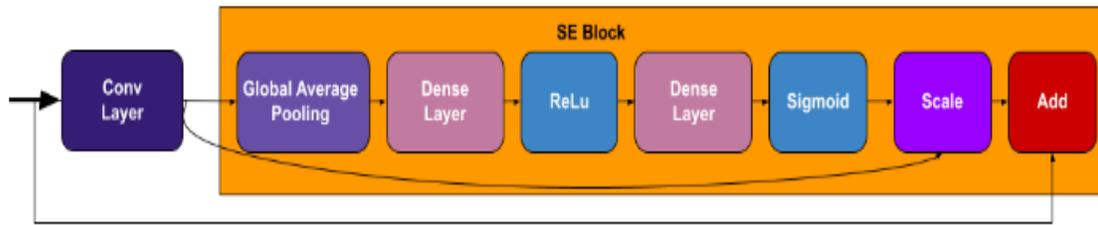
**Figure 4.8:** The squeeze and excitation (SE) block architecture
