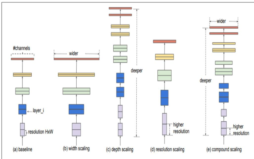
Figure 4.5: Scaling models.
