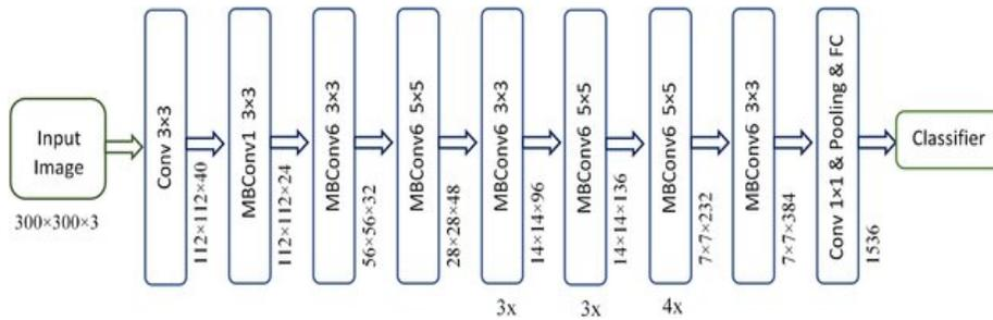
Figure 5.16: Architecture of EfficientNet B3
