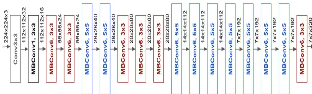
Figure 4.6: The EfficientNet-B0 architecture.
