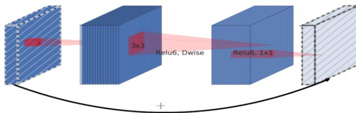
Figure 4.7: The structure of an inverted residual block (MBCConv)
