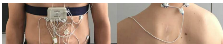
Figure 2.12: Placement of the RespiBAN and the ECG, EDA, EMG, and TEMP sensors. [55]
