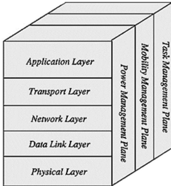
Figure 1.4: WSN Architecture [A. A. A. Alkhatib and Baicher \(2012\)](#)
