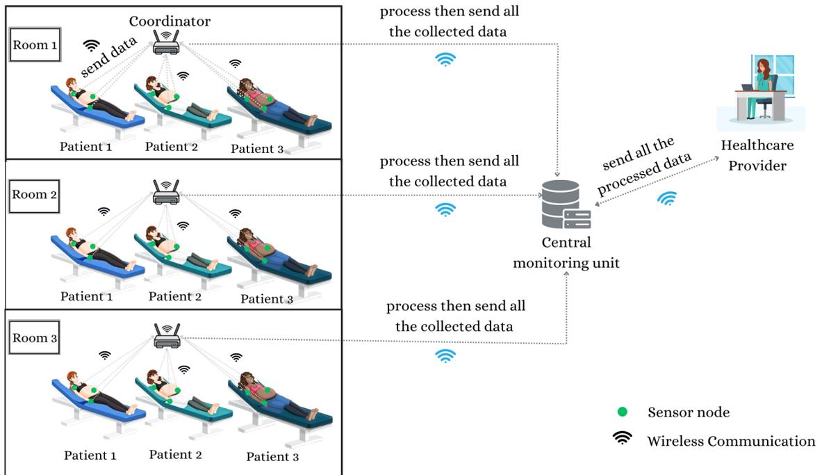
Figure 3.10: Semi-Centralized Data Processing in the Second Scenario
