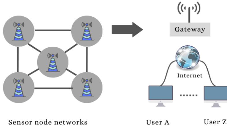
Figure 1.3: Wireless Sensor Network (WSN)
