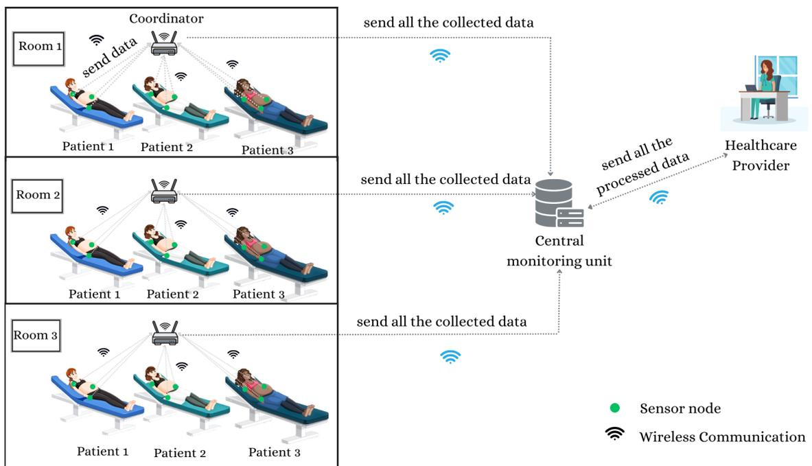
Figure 3.9: Centralized Data Processing in the First Scenario
