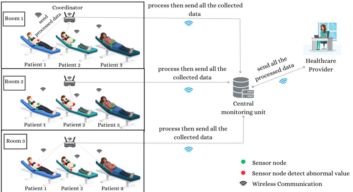
Figure 3.11: Decentralized Data Processing in the Third Scenario
