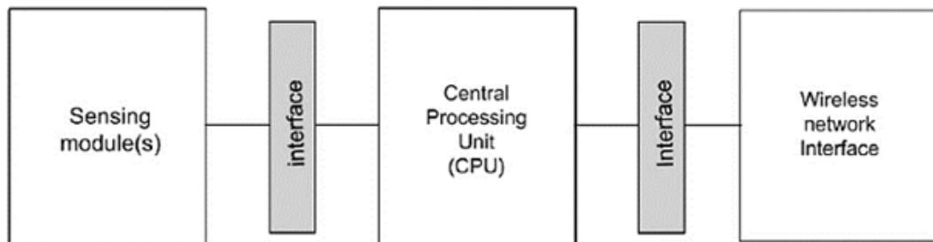
Figure 1.1: The Anatomy of a Sensor Node Bar-Noy et al. (2005)
