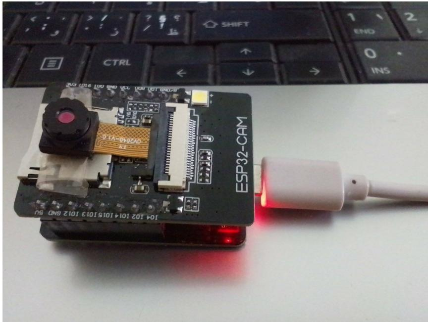
Figure 3.10: Connect the ESP32-cam with USB
