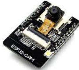
Figure 3.8: ESP32-CAM.
