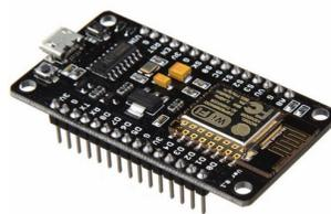
Figure 19: NodeMCU ESP-8266 board
