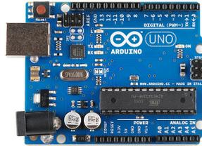
Figure 17: Arduino Uno Board
