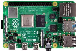
Figure 18: Raspberry Pi Board
