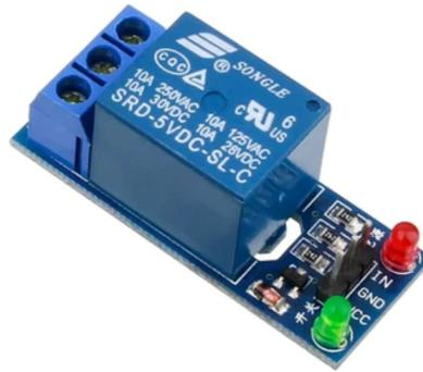
Figure 27: 2-Channel 5v Relay module
