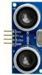
Figure 25: Ultrasonic Sensor HC SR-04
