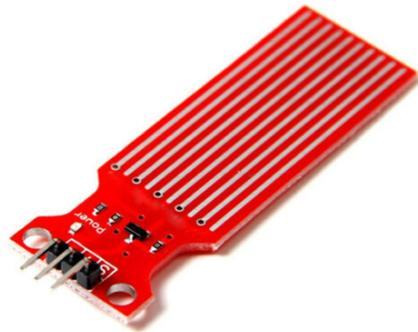
Figure 8: Water depth sensor
