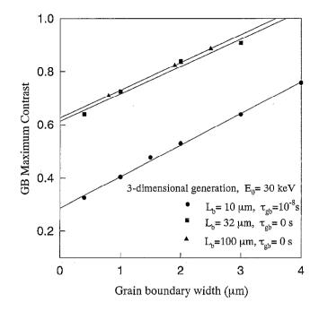
Fig. 5. Variation of the maximum EBIC contrast for different values of the bulk diffusion length and GB lifetime.
