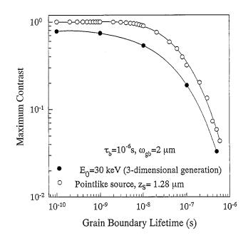
Fig. 2. Variation of the EBIC contrast vs. the carrier lifetime within the grain boundary.
