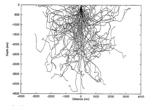
Fig. 4. Electron trajectories in Ge for a 30 keV beam. The beam size is taken equal to zero.
