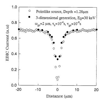
Fig. 1. EBIC contrast profiles across a 2 µm width grain boundary.
