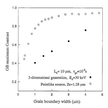
Fig. 3. Variation of the maximum EBIC contrast vs. the grain boundary width.
