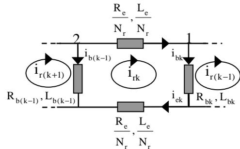
Fig.3. Electric diagram equivalent of a rotor mesh
