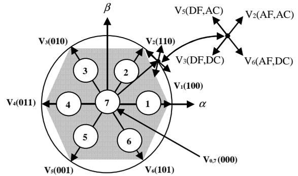
Fig 4: Partition of the complex plan in six angular
