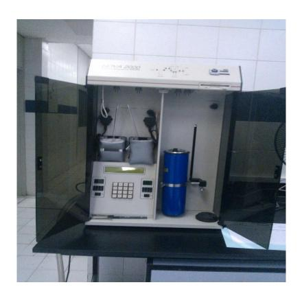
Figure III.6. Appareil Quantachrome NOVA 2200.
