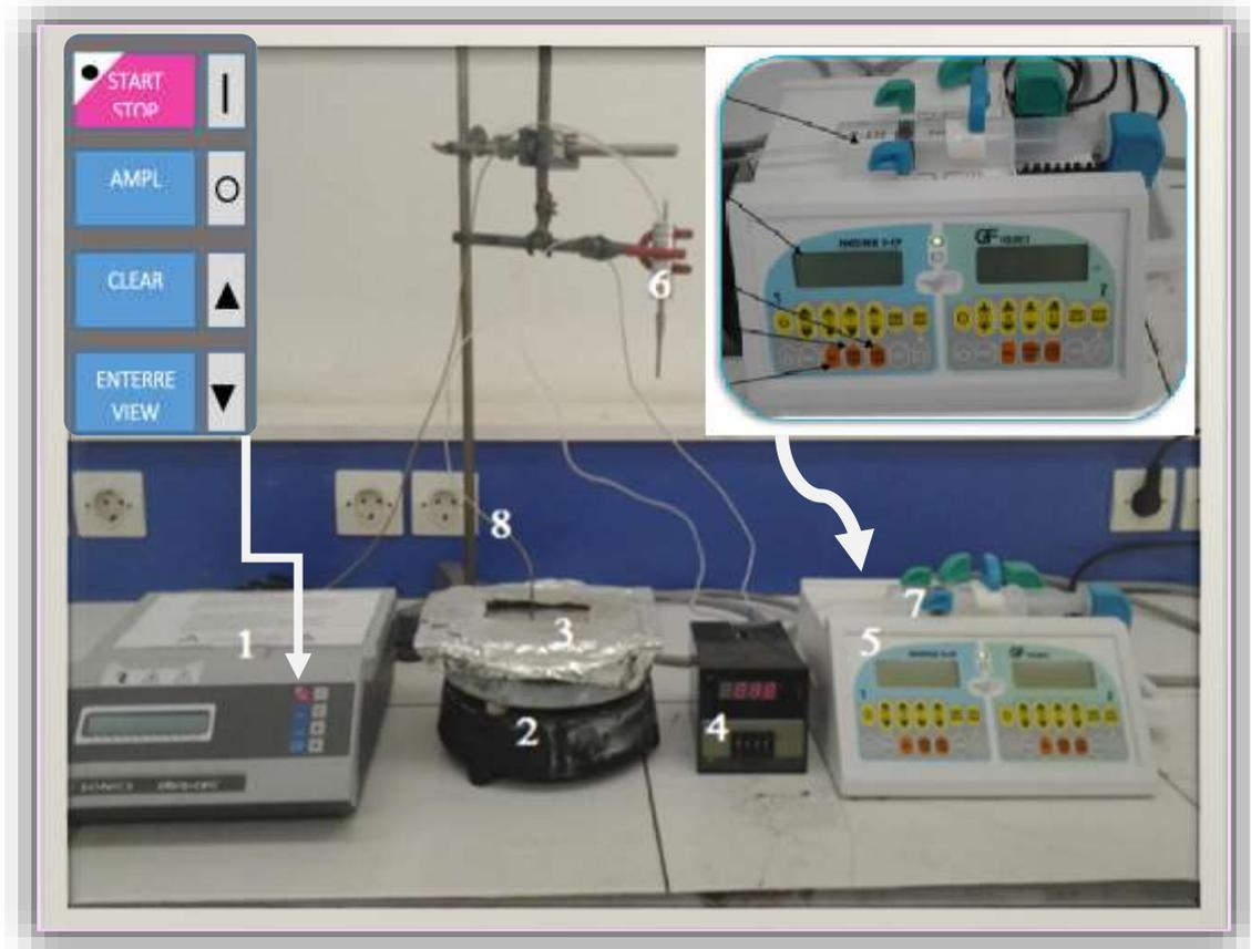
**FigII.2.** ultrasonic spray technique setup that used.
