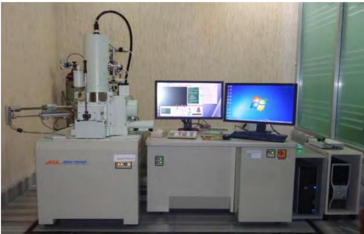
**Figure II.5:** Scanning electron microscope with EDS set up
