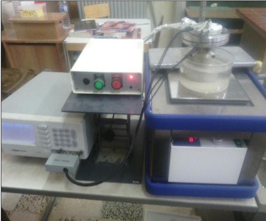
**Fig II.11:** GWINSTEK impedance meter, LCR- 821.
