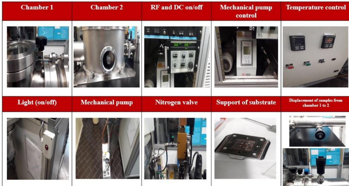
Figure 4.5: Sputtering detailed which used in this work.
