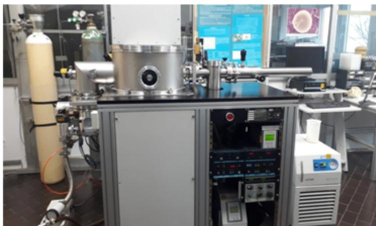
Figure 4.4: Sputtering is used in this work.
