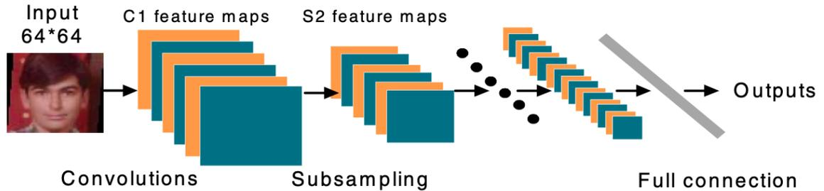
Figure 3.16: Yang et al [147] Convolutional neural network of 5 layers.
