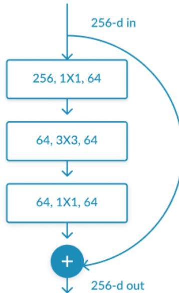
Figure 3.13: ResNet skip connection
