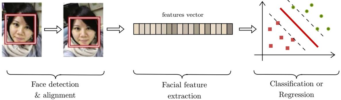
Figure 3.1: Typical pipeline of automatic facial soft biometric extraction systems. It consists of three phases: face face detection & alignment, facial feature representations and classification or regression.
