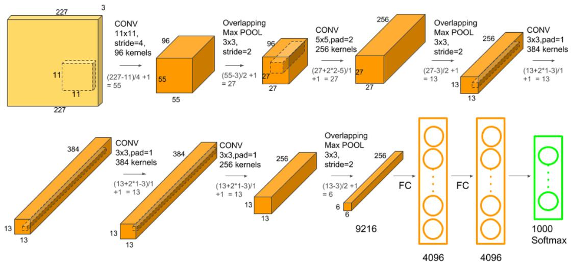
Figure 3.10: AlexNet architecture
