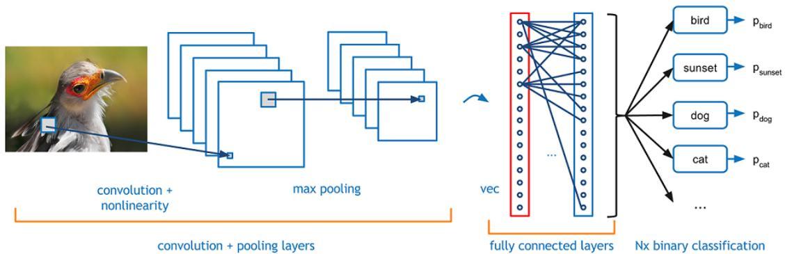
Figure 3.9: A general structure of a convolutional neural networks.
