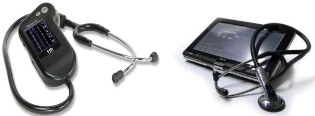
**Figure (1.6).** *The DigiScope Collecto hardware prototype. It has unrivalled acoustic performance of 24x magnification with 85 percent of the noise reduction for friction and ambient noise.*
