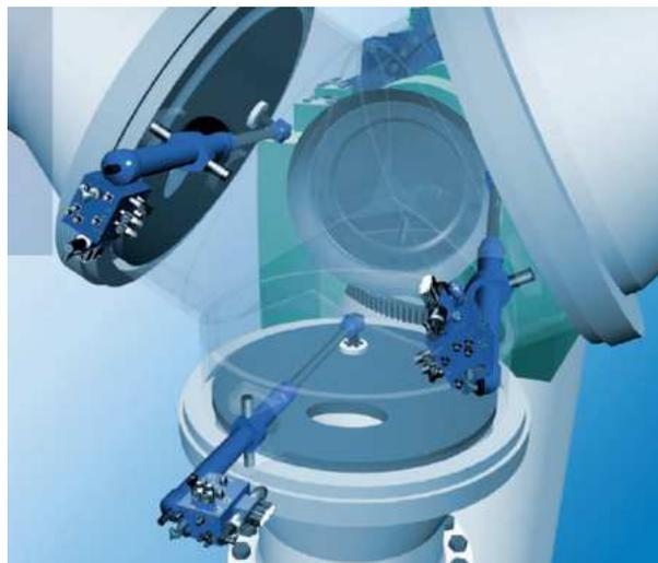
**Figure 2.8** Hydraulic blade pitch control system [14].
