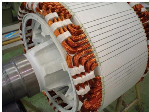
**Figure 1.12** Wounded rotor used in the DFIG.
