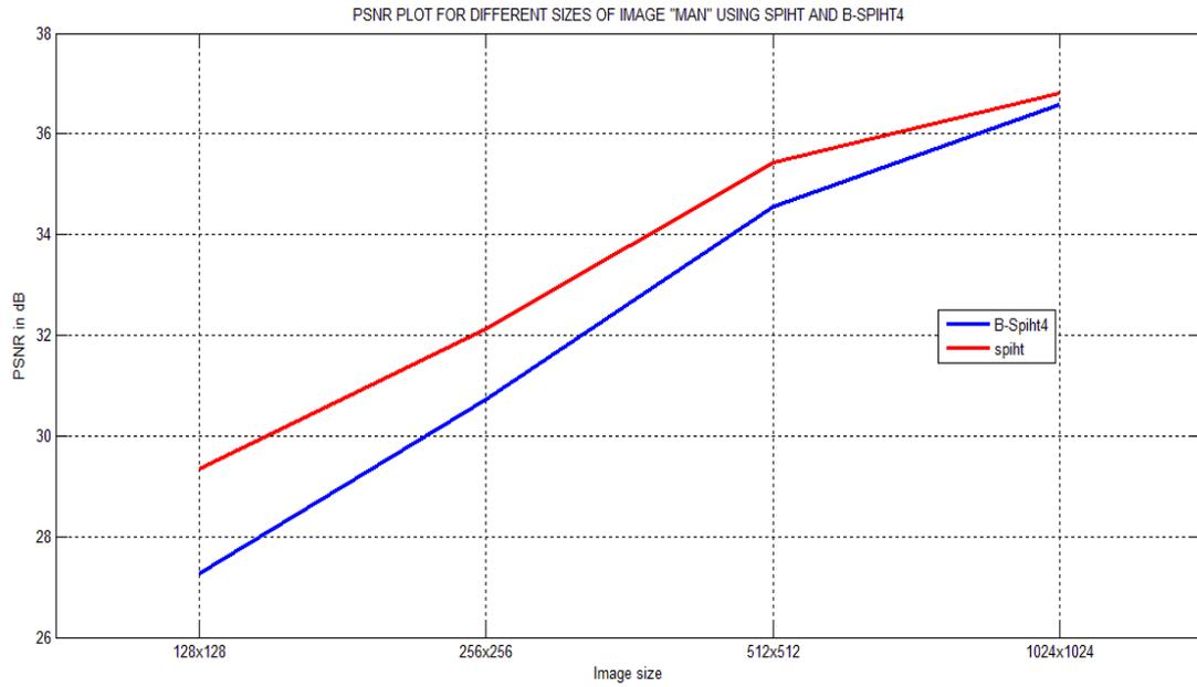
Figure 4.43: PSNR of SPIHT and B-SPIHT for different sizes of image man at 1bpp
