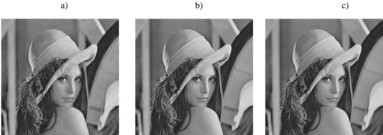
figure 4.36: visual quality for SPECK a) 0.1 bpp, 29.57 dB, b) 0.42 bpp, 36.09 dB, c) 1.72bpp, 43.68 dB
