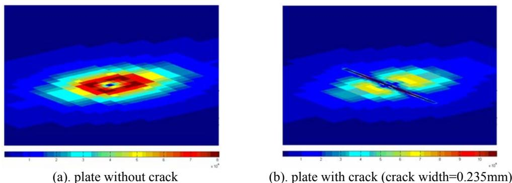
Fig.3. Eddy currents density colormap on the top surface of the conductive plate of JSAEM#6 problem
