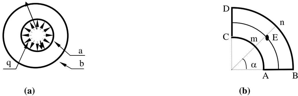
**Fig.2.6: Thick cylinder under internal pressure.**
