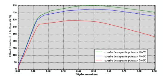
Fig4.39: Courbe de capacité -SeismoStruct -Lp=0.08L+0.022FY.db
