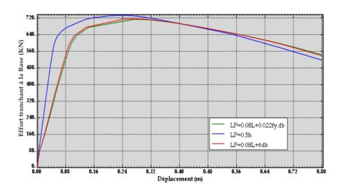
Fig4.35: Courbe de capacité-SeismoStruct —Poteaux 50x40
