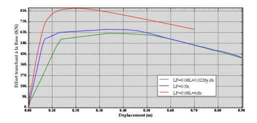
Fig4.46: Courbe de capacité-SeismoStruct –Poteaux 50x50
