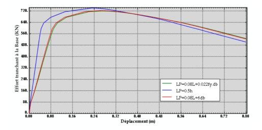
Fig4.36: Courbe de capacité-SeismoStruct —Poteaux 50x50
