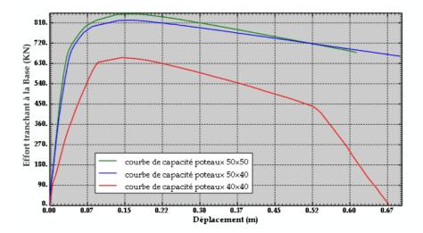
Fig 4.18: Courbe de capacité-SeismoStruct - LP=0.5h
