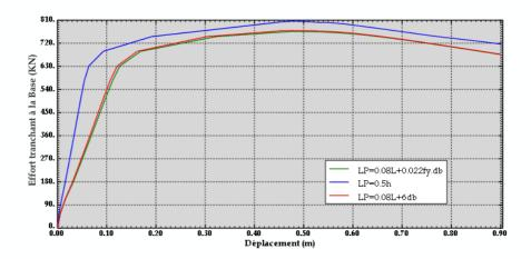
Fig4.45: Courbe de capacité-SeismoStruct —Poteaux 70x50
