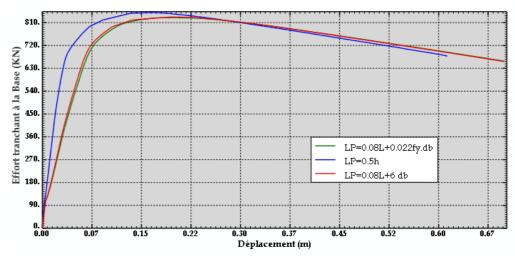
Fig 4.25: Courbe de capacité-SeismoStruct -Poteaux 50x50
