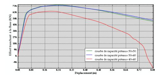
Fig4.29: Courbe de capacité-SeismoStruct - LP=0.5h
