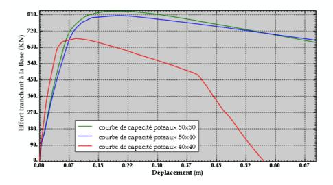
Fig 4.17: Courbe de capacité -SeismoStruct -Lp=0.08L+0.022FY.db
