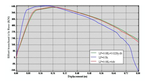
Fig4.34: Courbe de capacité-SeismoStruct –Poteaux 40x40
