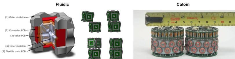
**Figure 2.17:** Fluidic assembly and *Catom* robots
