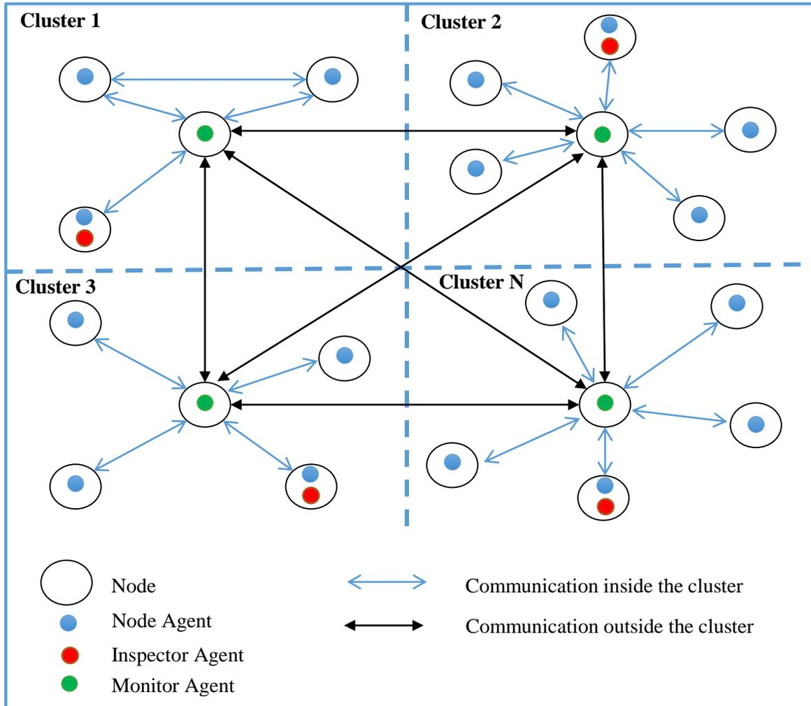
**Fig 5.1: Our proposed architecture for security Model based Mobile Agent in MANETs**
