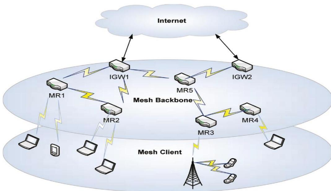
Figure 2.4: A typical Architecture of a WMN
