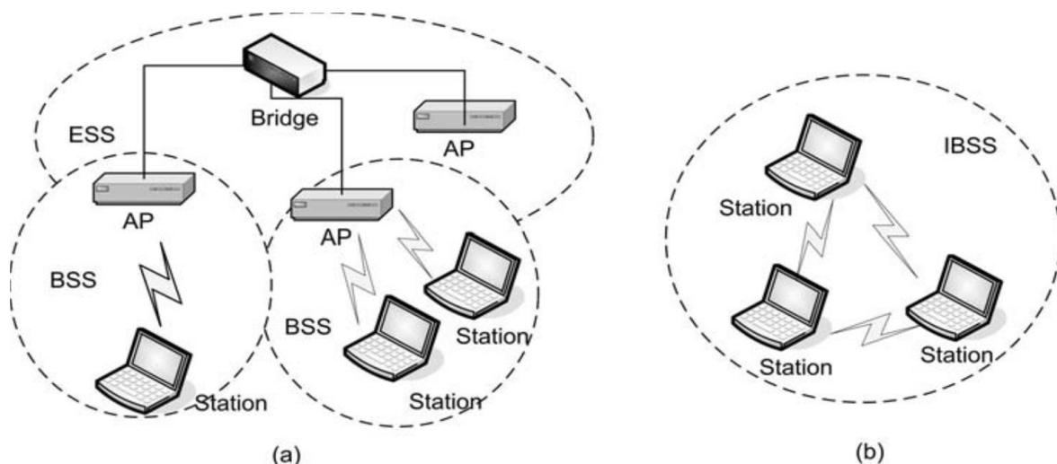
**Figure 2.2: Illustration of WLAN Configuration: (a) ESS Composed of Infrastructure BSS, and (b) IBSS [28]**
