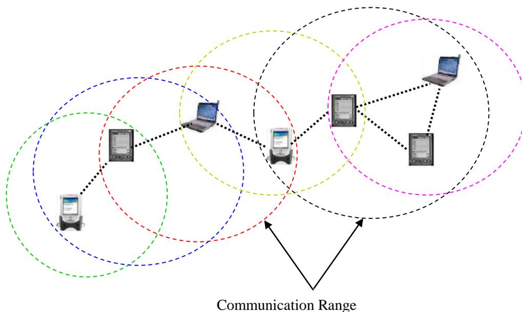
**Figure 2.5: Illustration of Mobile Ad Hoc Networks**
