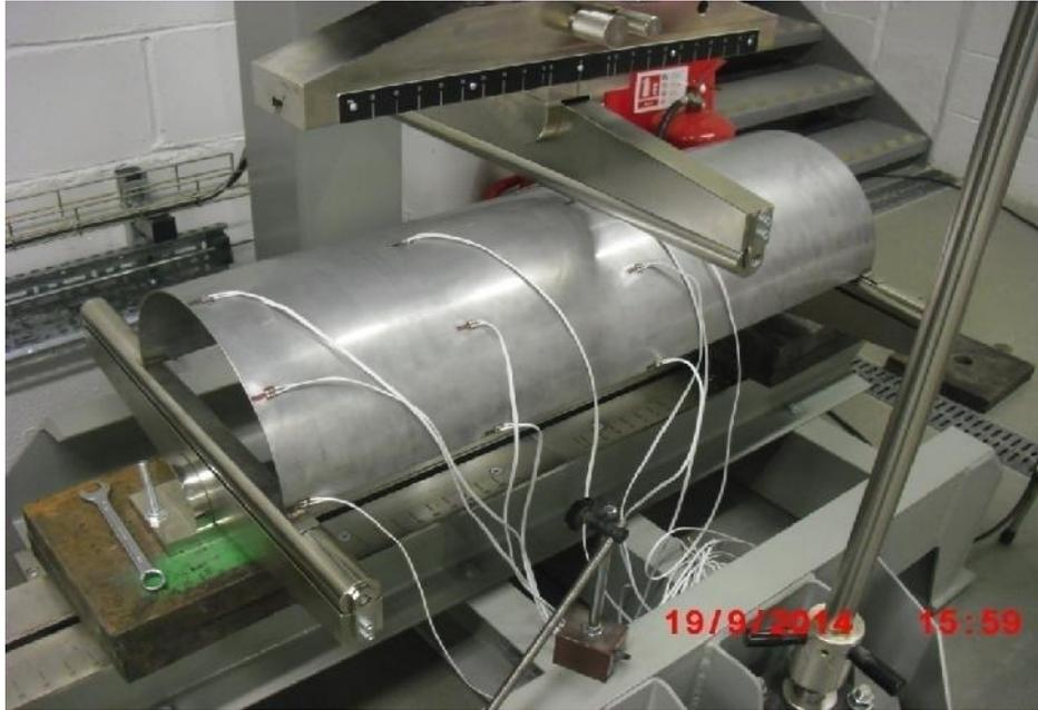
**Fig. 3.2** The specimen on UNIFLEX 300 machine
