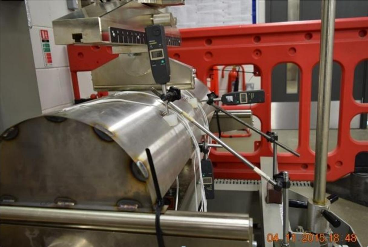
Fig. 5.7 Cylindrical shell model with rigid diaphragm and stiffeners undergoing the loading
