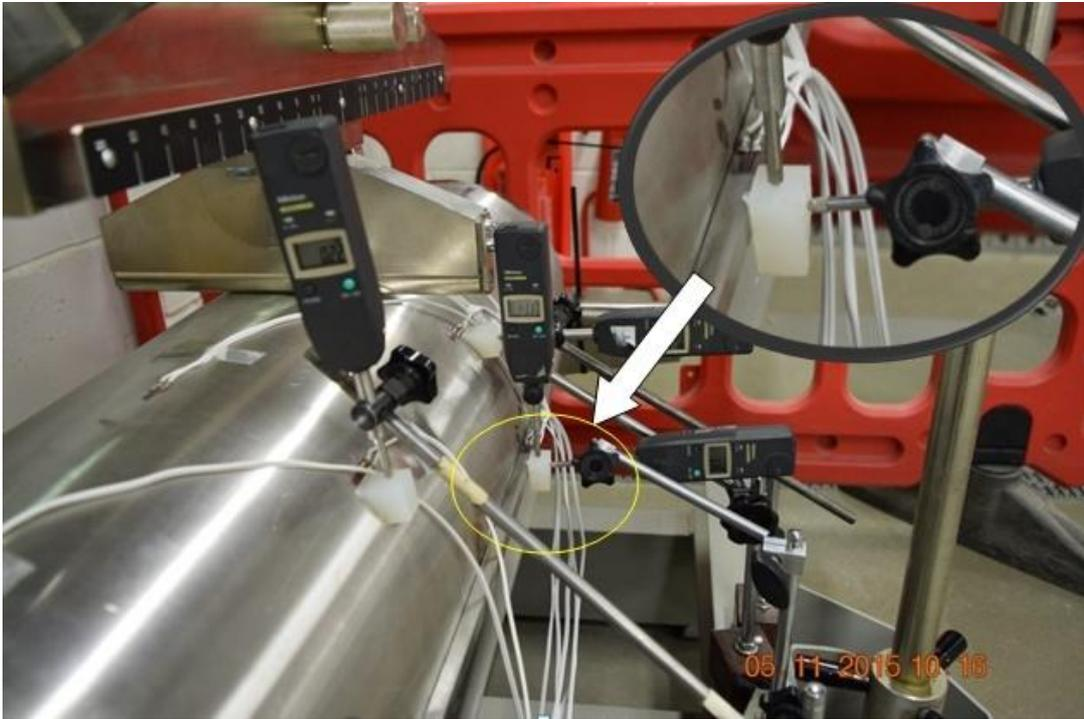
Fig. 3.14 Dial gauges positioning, and applied loading
