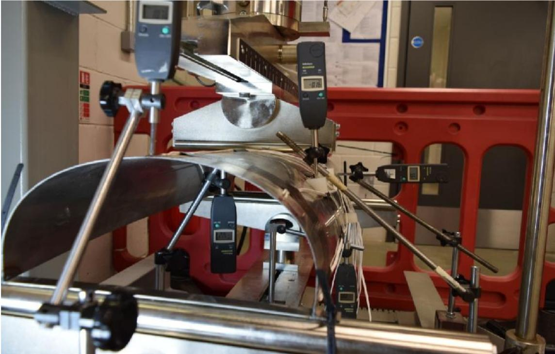
**Fig. 4.7** Cylindrical shell model undergoing the loading
