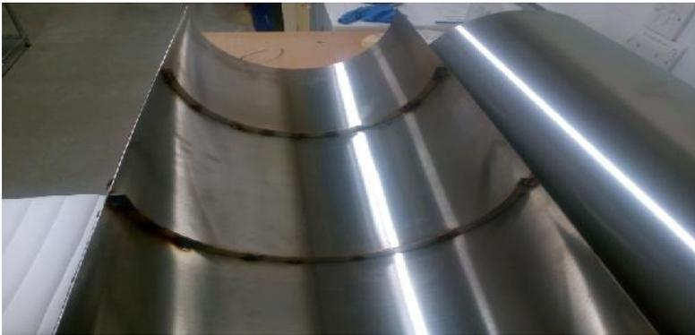
**Fig. 3.5** Cylindrical shell with two stiffeners
