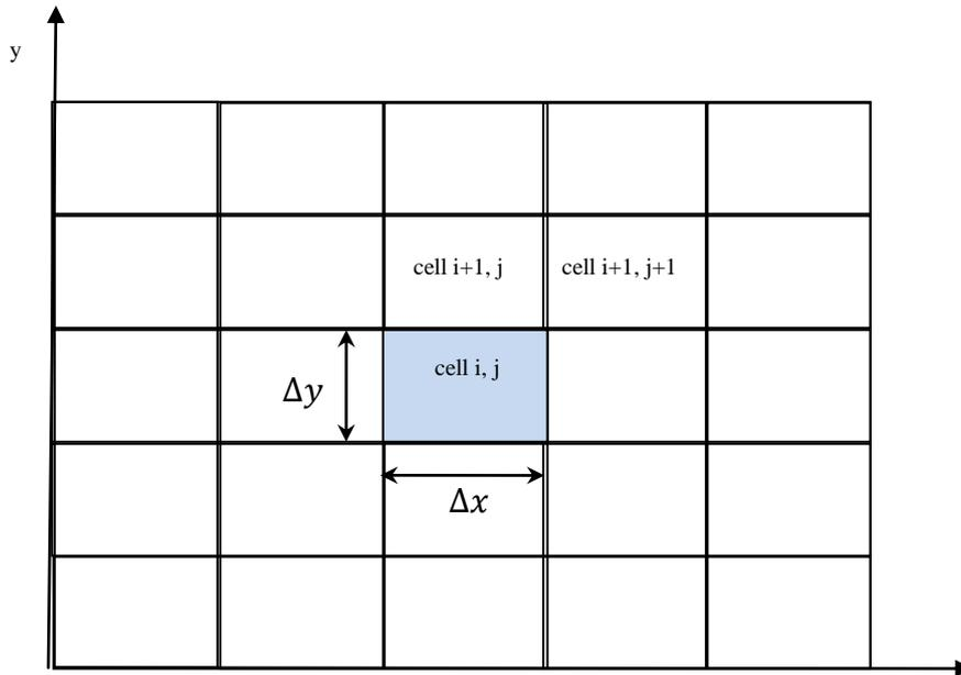
Figure 5. 3 Two-dimensional grid.
