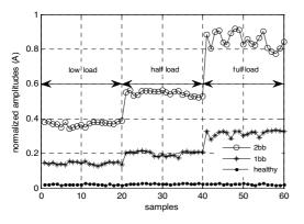
Fig. 5. Normalized amplitudes of the  $f_{bb}$  harmonics for: healthy rotor, one and two broken bars. First classification.
