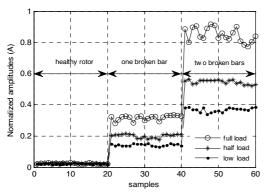
Fig. 6. Normalized amplitudes of the  $f_{bb}$  harmonics for the three rotors: healthy, one and two broken bars. Second classification.
