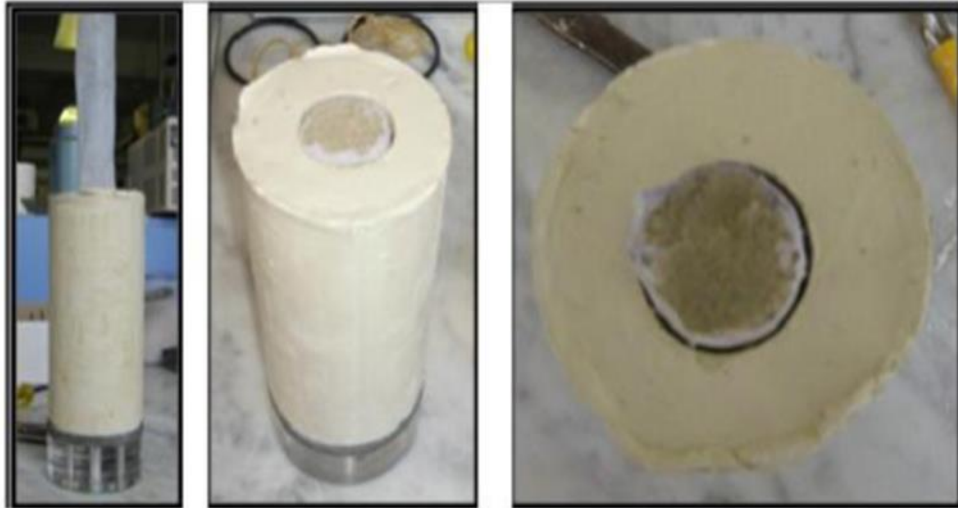
Figure 2-28. Installation of encased sand (Najjar et al. 2010).
