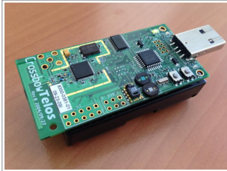
Figure I.1: A typical sensor node
