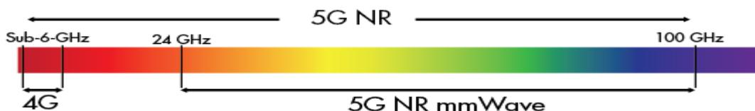
Figure 1.2. 5G New Radio frequency (5G NR): The mmWave.
