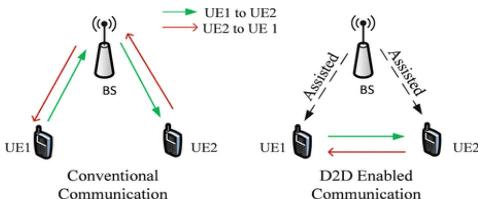
Figure 1.5. D2D communication and Conventional communication.
