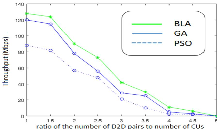
Figure 3.6. Impact of increasing ratio of D2D pairs number to CUs number with rate requirement of 250kbps for each user.
