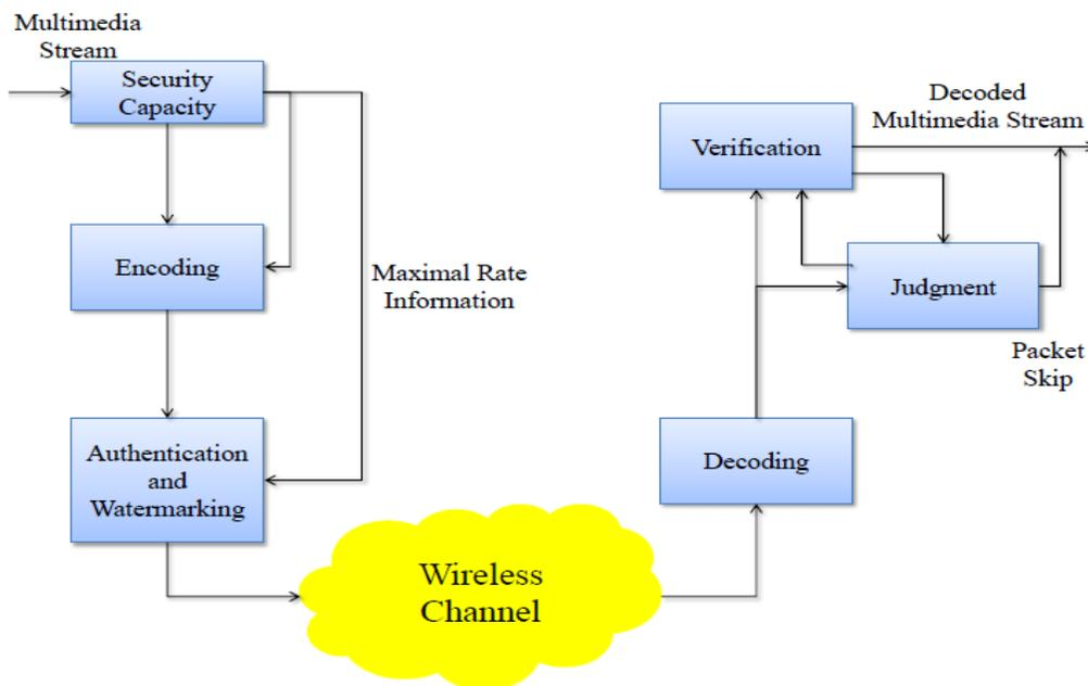
Figure 1.13. Combined Physical-Application Layer Security Scheme
