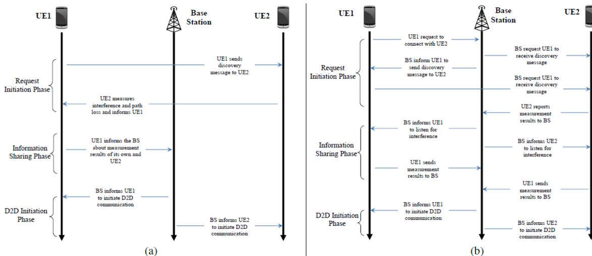
Figure 1.10. Centralized device discovery (a) Partial involvement of BS, (b) Complete involvement of BS.
