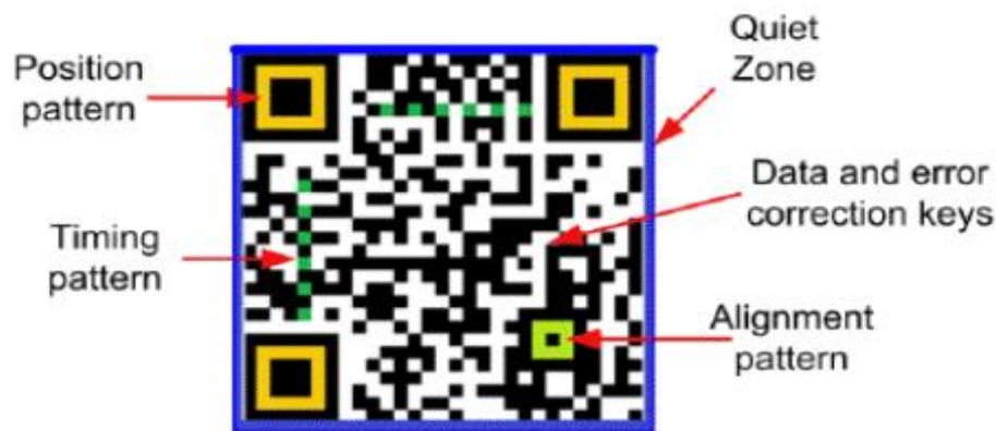
Figure 2.2 : Components of QR code
