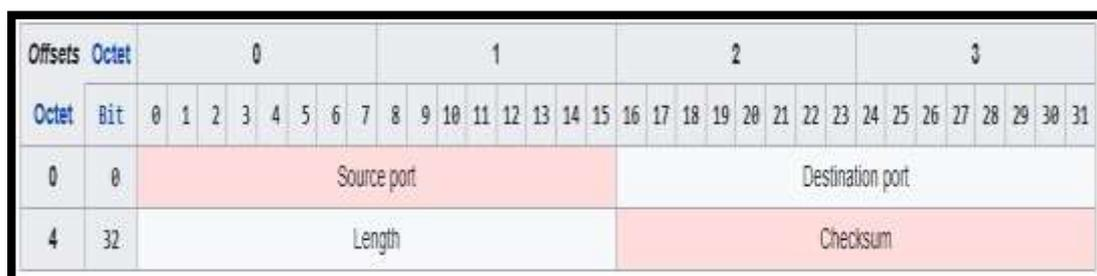
Figure II 5 : Diagram of UDP datagram header
