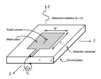
Figure 2.1:Geometry of a Rectangular Microstrip Antenna.
