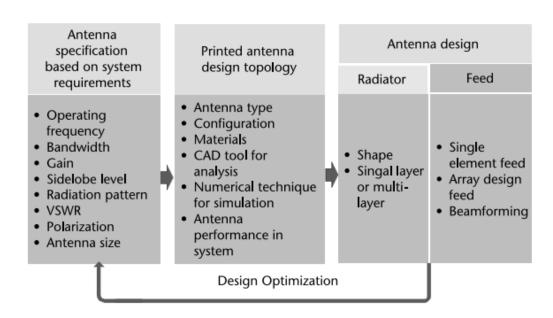
Figure 3.1 Microstrip patch antenna design flow
