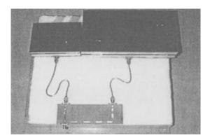
Figure 2.17:Photograph of Ultra-wideband Printed Antenna
