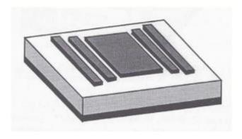
Figure 2.12: Parasitic microstrip antenna patch
