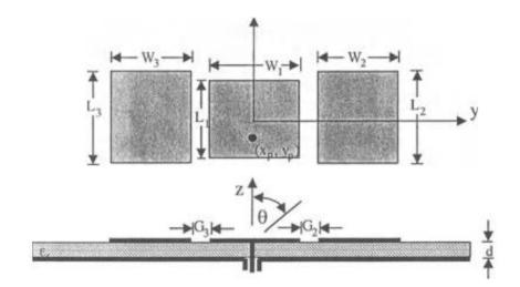
**Figure 2.11:Horizontal Parasitically Coupled Patches**
