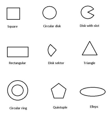
Figure 1.2: Antenna patch types
