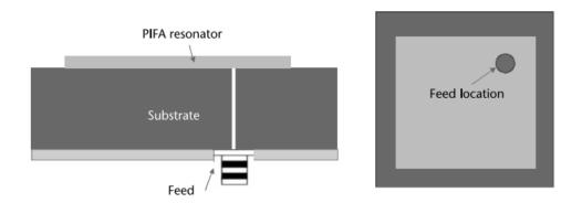
Figure 2.8 Coaxial-fed microstrip patch antenna (side and top view)
