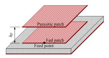
Figure 2.13:Stacked Microstrip Antenna
