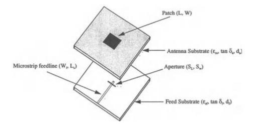
Figure 2.15:Large Slot Aperture Coupled Patch Antenna
