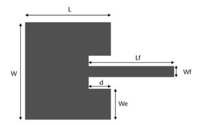
Figure 3.3:Inset fed rectangular microstrip antenna design
