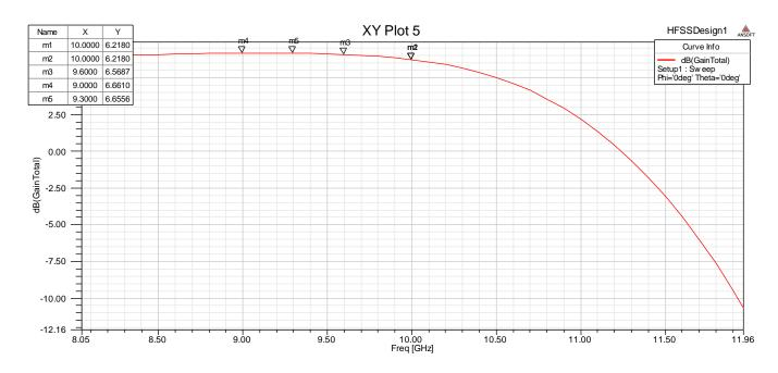
Figure 3.9: the Gain variation in terms of the Frequency
