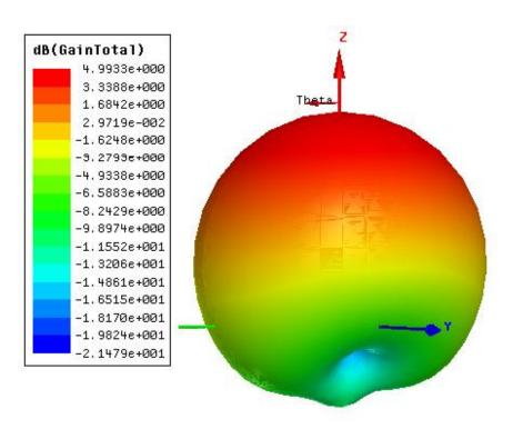
Figure 3.15:3d Polar Gain Plot
