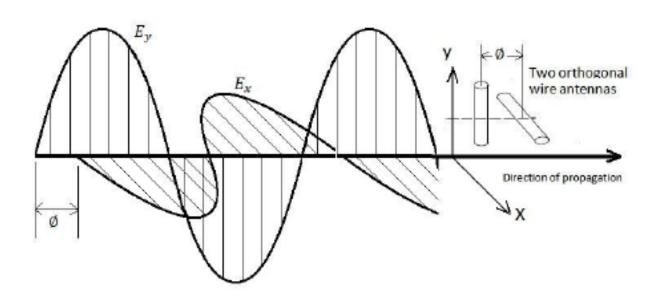
Figure 1.7:Polarization of electromagnetic wave
