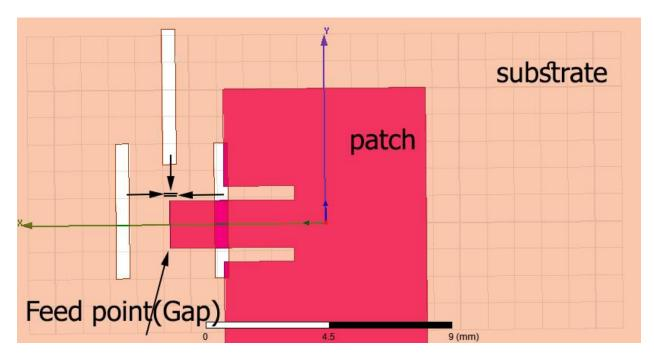
Figure 3.11: microstrip antenna with 3 slots in the ground plane
