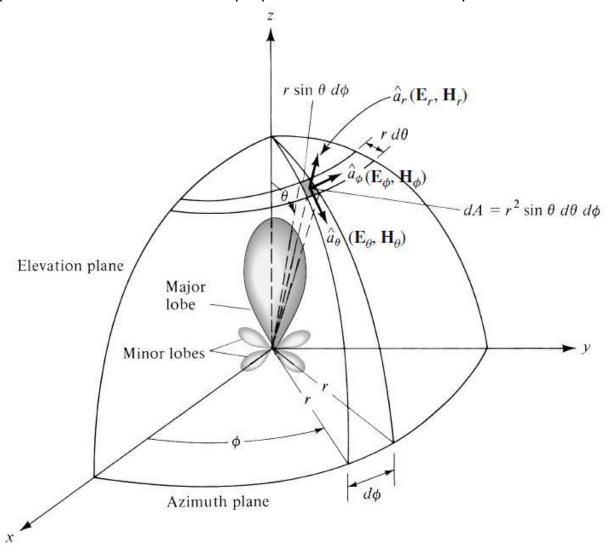
Figure 1.4: Radiation pattern graphical representation (1)
