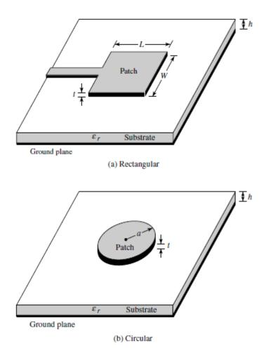
Figure 1.1: Patch antenna most used types
