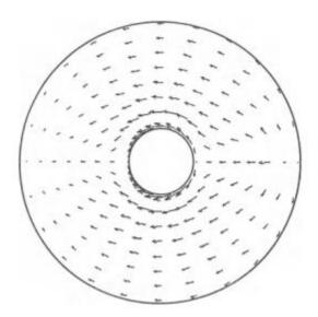
Figure 2.4:Typical CurrentslFields Excited on an Annular RingPatch
